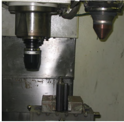
Figure 1: The LAMP process during a repair operation - The laser cladding head is shown on the right. A touch probe head is currently held in the machining spindle. A repaired H13 tool steel die component is held in the vise.
