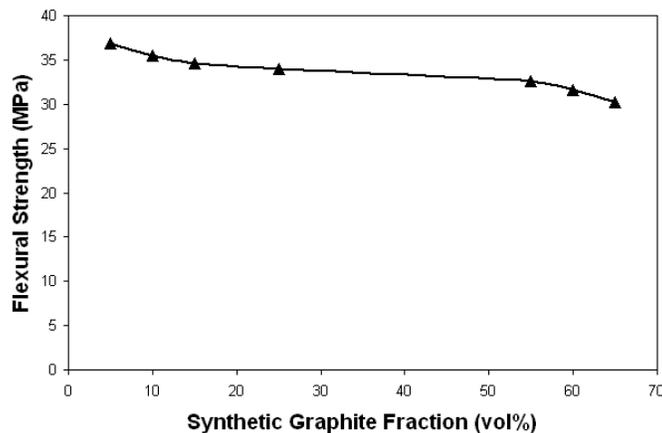
Fig. 4 Flexural strength varies with different SG fraction.
