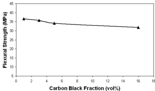
Fig. 10 Flexural strength varies with different CB fractions.
