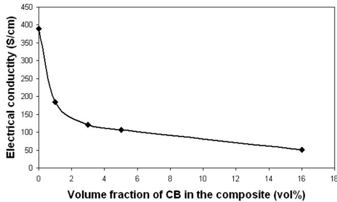
Fig. 9 Electrical conductivity varies with CB fractions.
