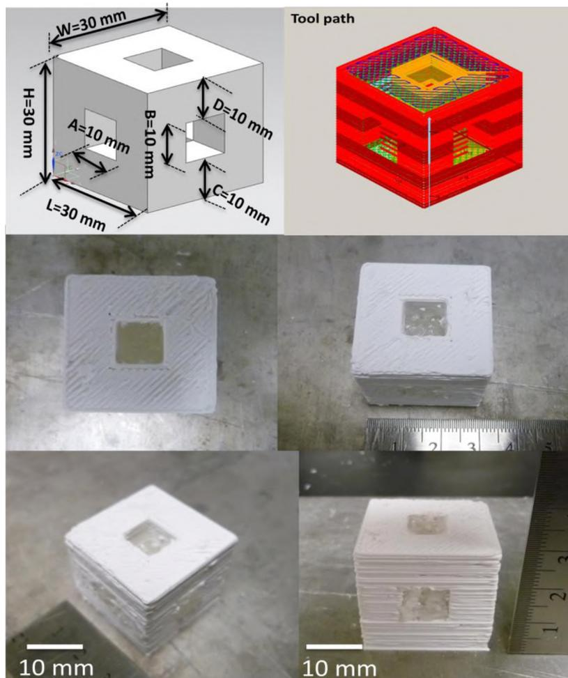
Figure 12. CAD model of a cube with a square hole on each side and the extruded part with sacrificial material
