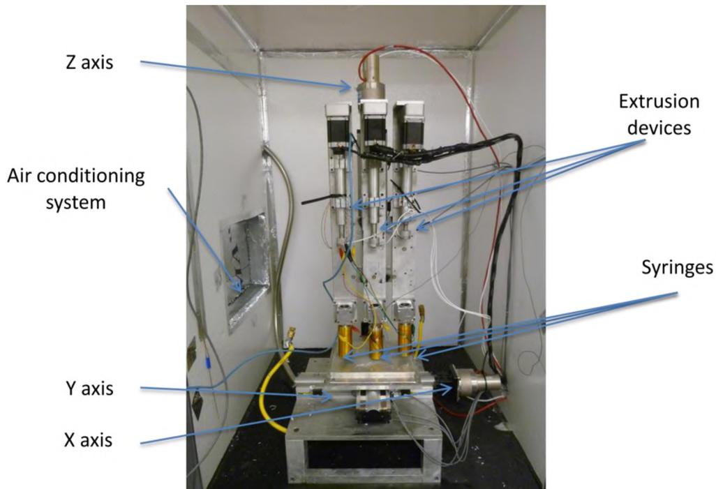
Figure 1. Experimental setup of the multiple-extruder FEF machine
