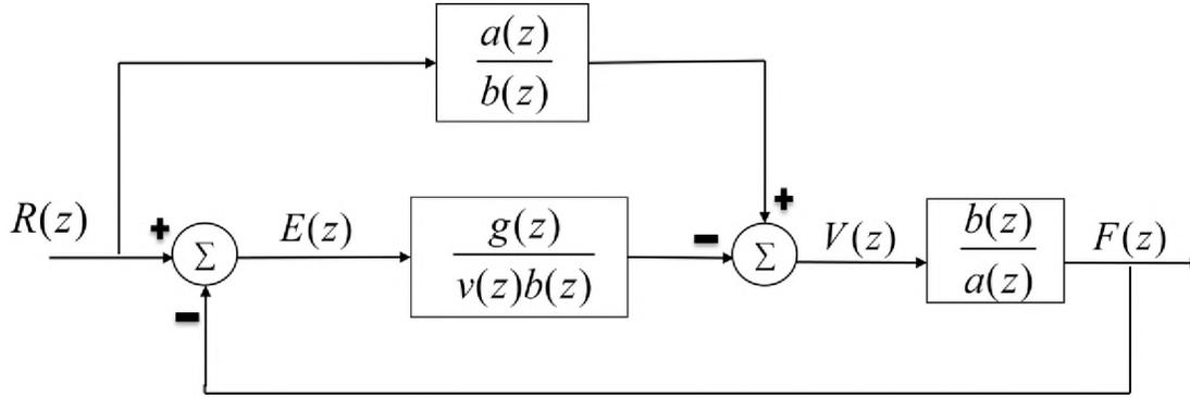
Figure 6. Block diagram of the general tracking controller
