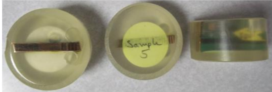
Figure D.10. Example of labeling the sample, and using plastic holders
