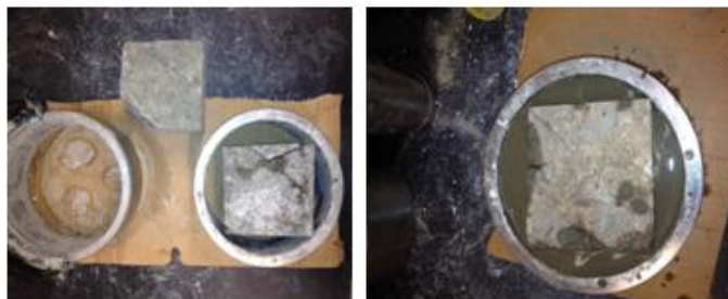
Figure 3-3. Cementing of the rock sample
