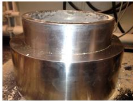
Figure D-6. Shear ring stuck inside the shear box
