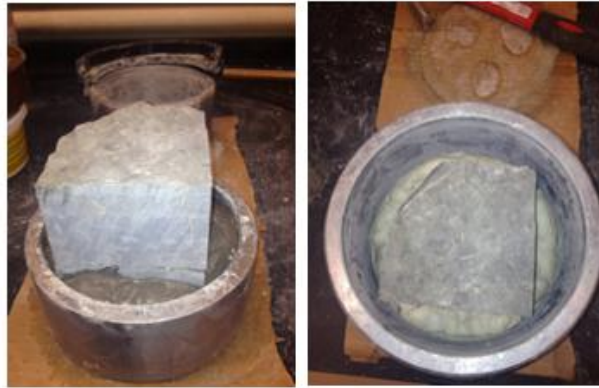
Figure 3-4. Rock sample inside the shear ring
