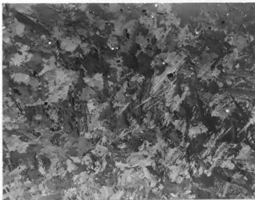
0.51 atomic per cent silicon 50X , polarized light
