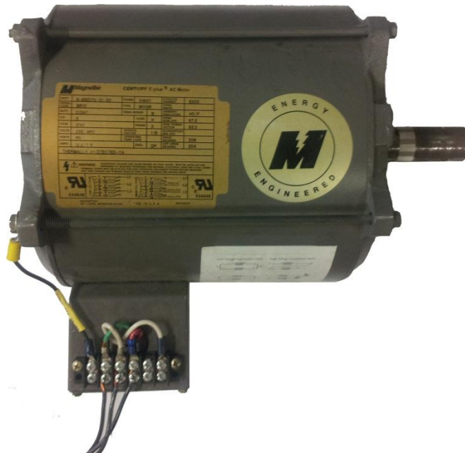
Figure A.7 Induction Machine – II Load
