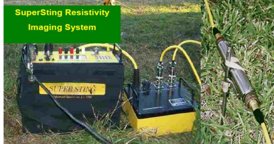
Figure 6.6. Earth resistivity meter-SuperSting R8/IP, manufactured by Advanced Geosciences Inc.
