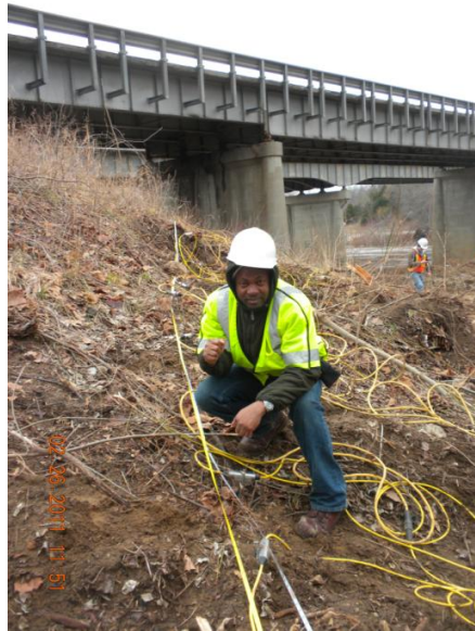
Figure 1.2. Data acquisition of ERT at the site and the nature of the site
