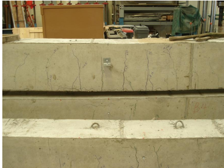
Figure 4.10. Failure of Beam 1
