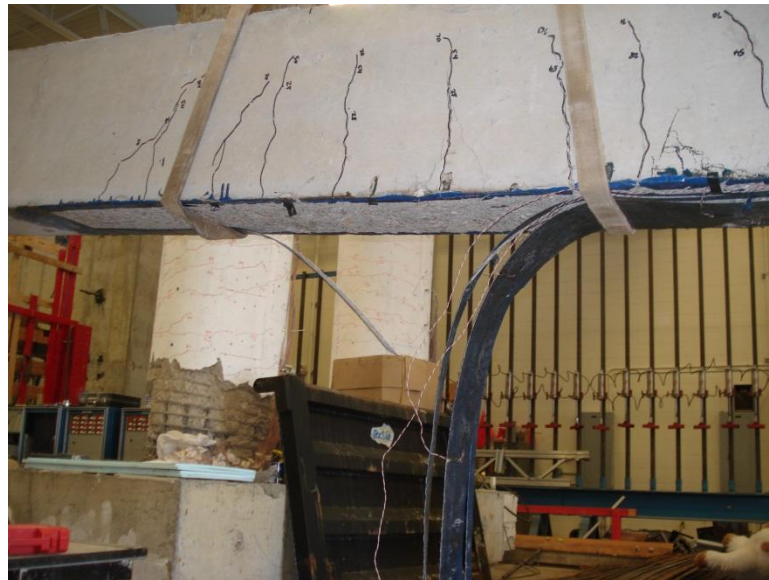
Figure 4.37. Failure of Beam 3
