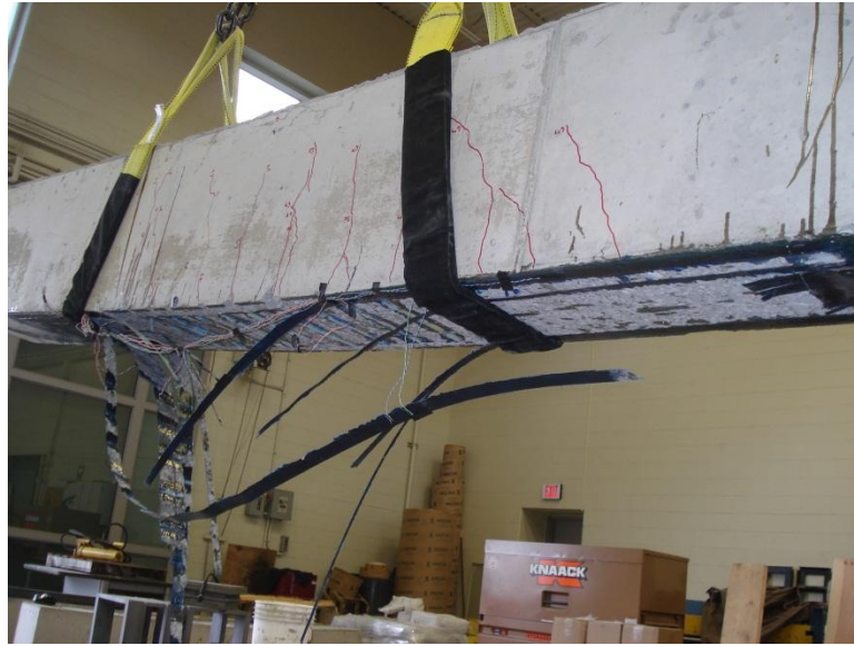
Figure 4.67. Failure of Beam 10
