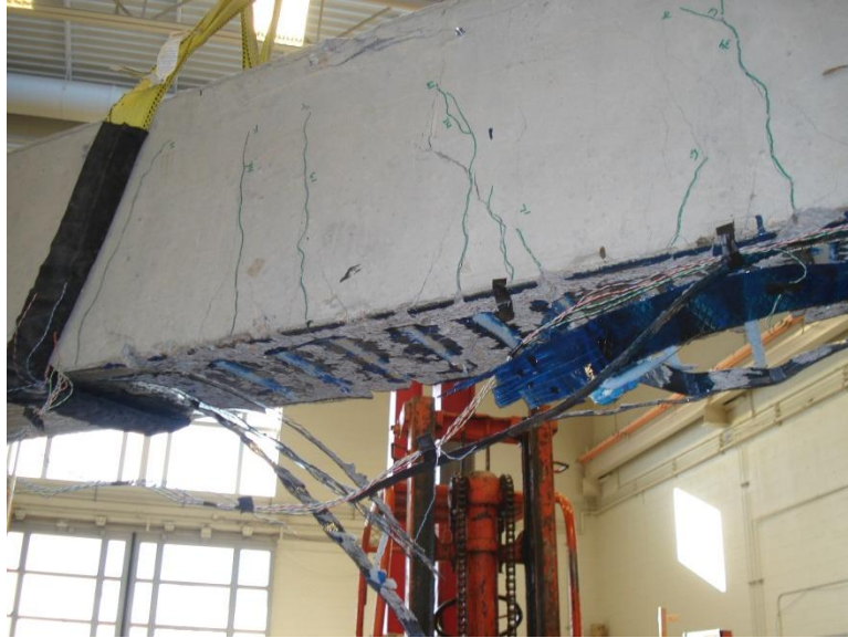
Figure 4.51. Failure of Beam 6
