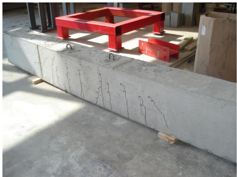
Figure 4.31. Failure of Beam 1
