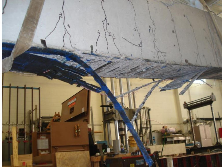
Figure 4.41. Failure of Beam 4
