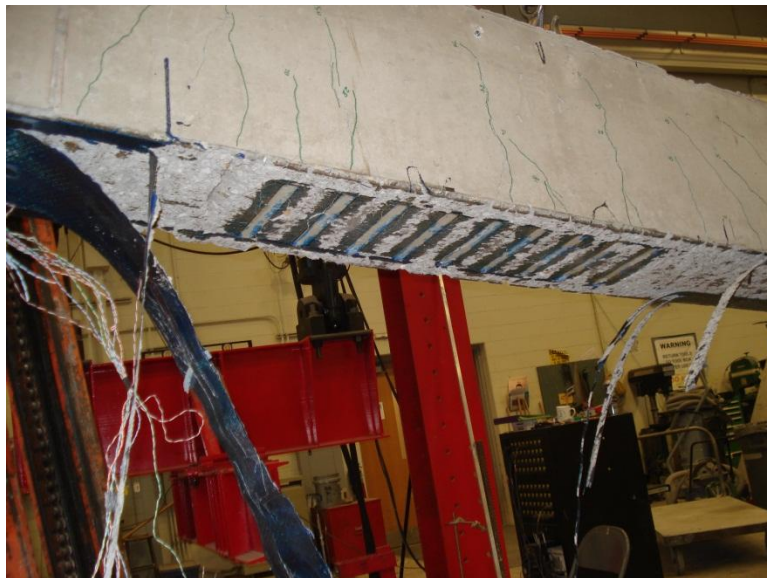
Figure 4.56. Failure of Beam 7
