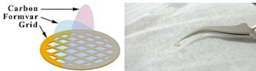
Figure 4.6. Schematic steps for sample preparation for STEM/TEM.
