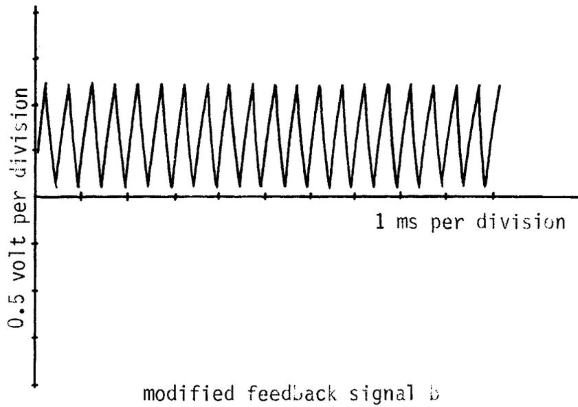
Figure 6. Modified Signal (1000 Hertz Input)
