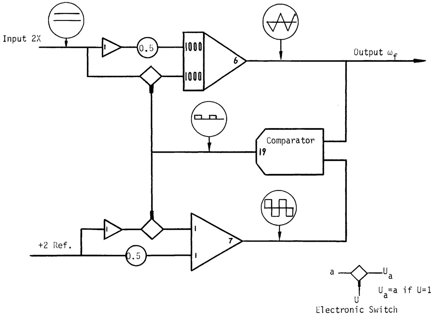
Figure 3. D.C. Level to Frequency Converter Circuit
