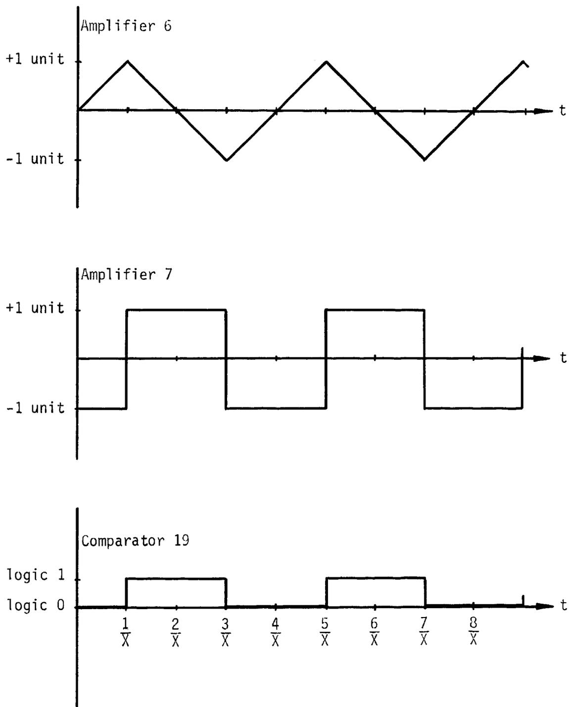
Figure 4. Waveshapes for D.C. to Frequency Converter
