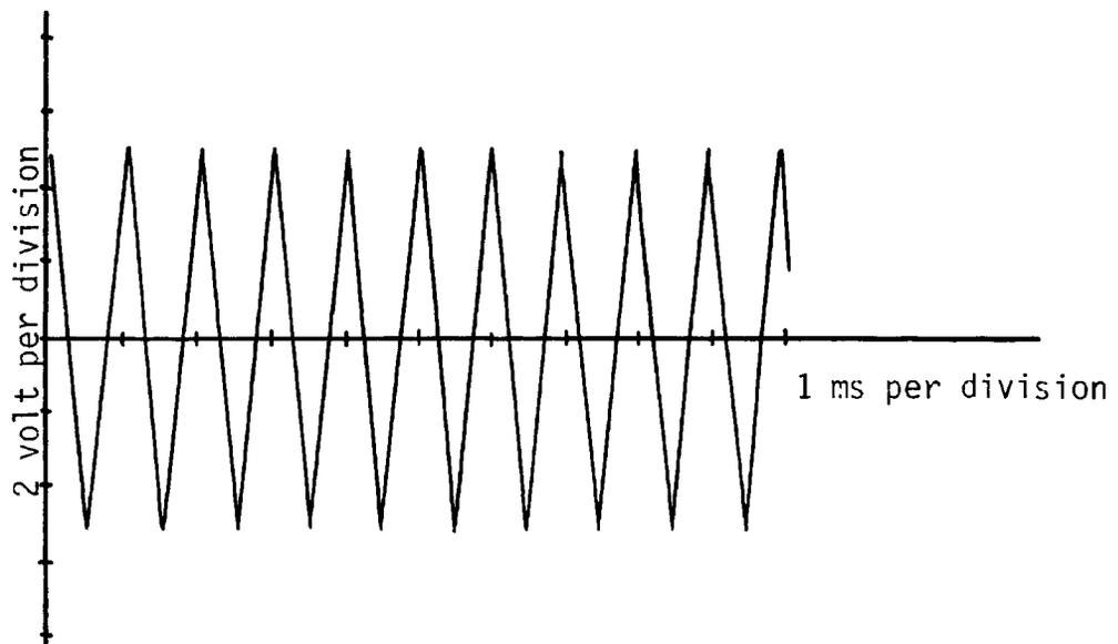
Figure 8. Output of D.C. Level to Frequency Converter
