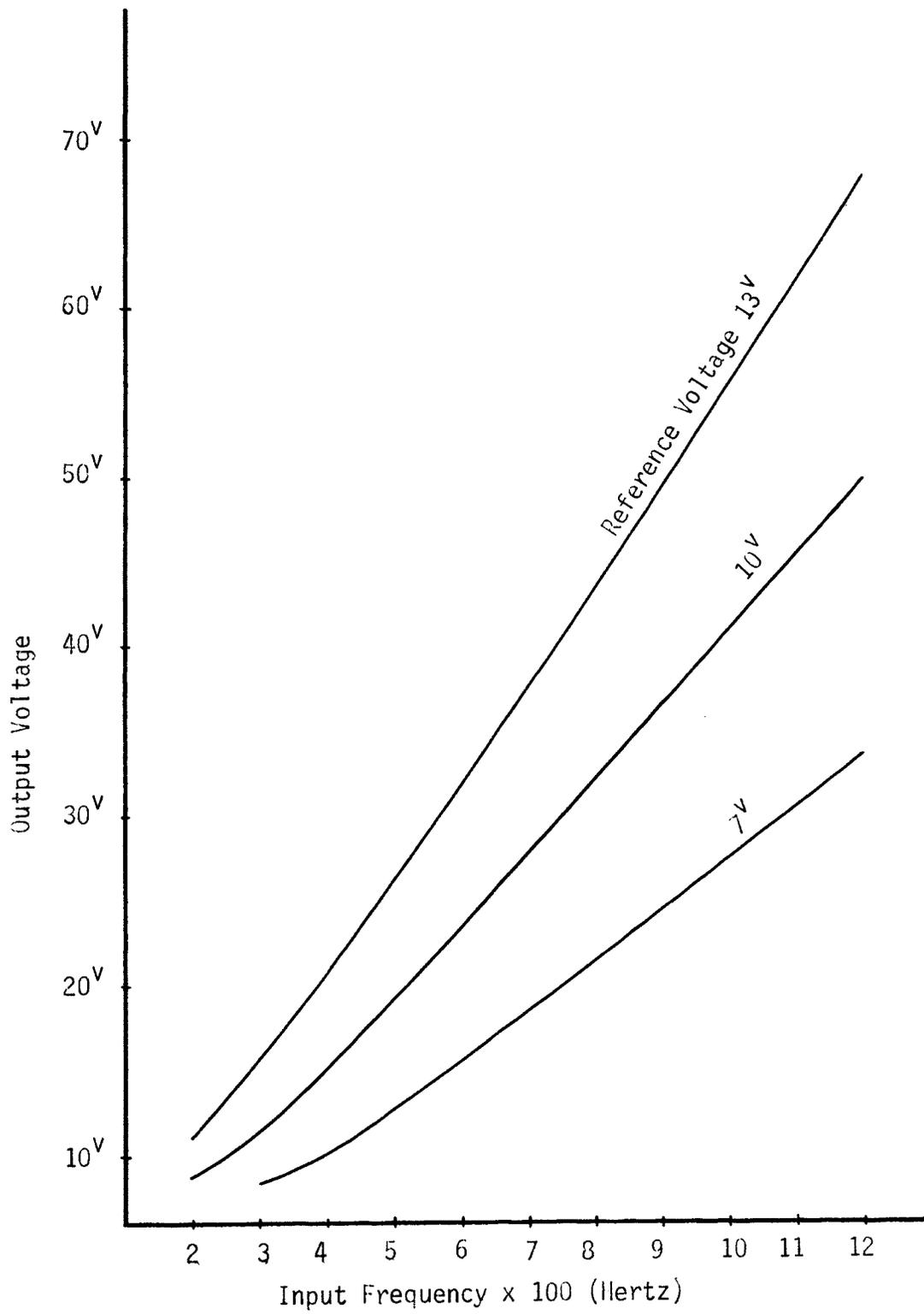
Figure 10. Steady State Response of Overall Measuring System
