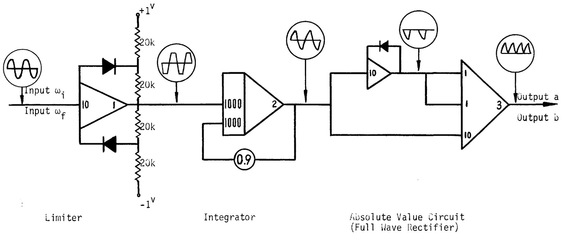
Figure 2. Limiter, Integrator and Absolute Value Circuit
