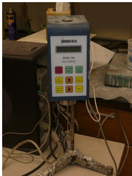
Figure 2.2 Brookfield DV-II+ Pro viscometer used to measure slurry viscosity
