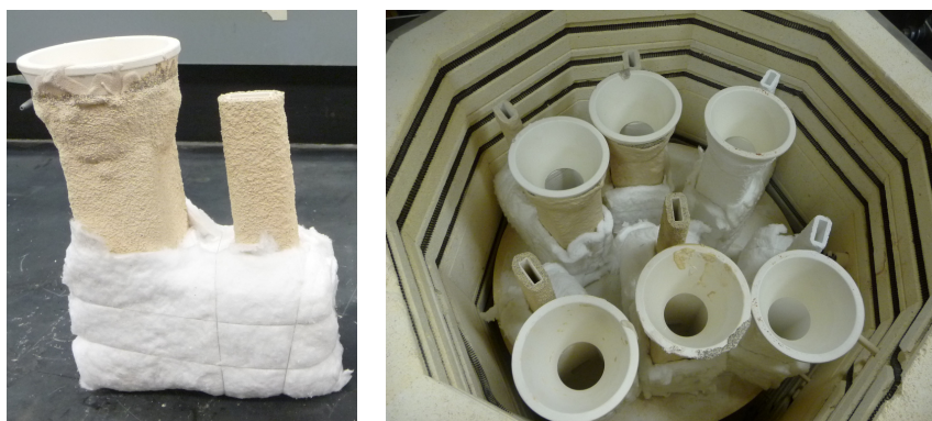
Figure 4.9 (a) Shells coated with kaowool and (b) preheating in kiln
