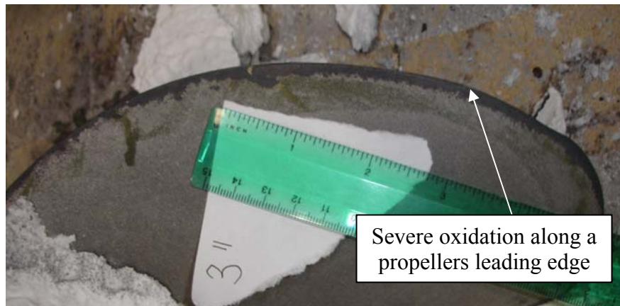
Figure 2.1. Oxidation along the leading edge of a cast marine propeller.
