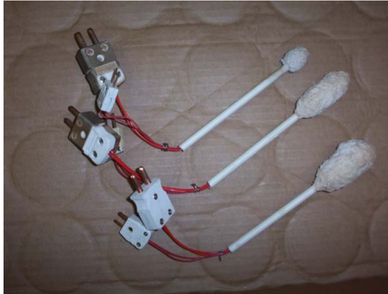
Figure A.7. Completed thermal conductivity probes.
