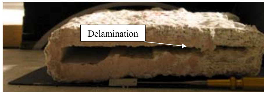
Figure 4.3. Investment shell exhibiting primary coat delamination.
