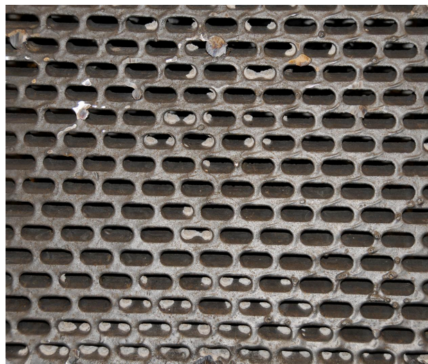
Figure 19. Section of bottom-filled P900 plate poured into a ceramic shell preheated to 800°C (1472°F) with a 180°C (324°F) superheat.
