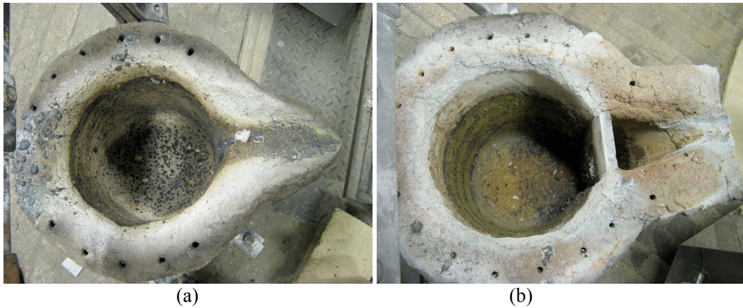
Figure 22. (a) Lip-pour ladle used for Heats 1-4 and (b) teapot ladle used for Heat 5.
