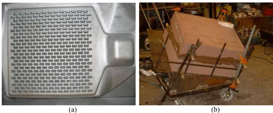
Figure 14. Drag-side of P900 match-plate (a) and 15° tilt sand mold on specially designed pouring cart (b).
