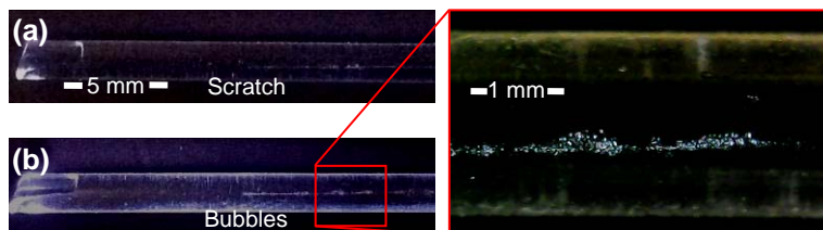
Fig. 3. Dark-field images of scratched filament (a) before and (b) after laser scanning
