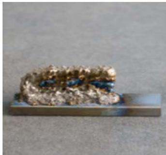
(a) Deposition with non-smooth zigzag toolpath
