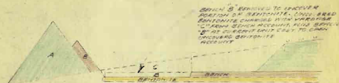
Bench Removed - Bentonite Uncovered
