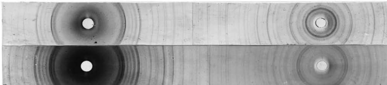
Figure 12. (above) The X-ray Powder Photograph of the Sample Contains 80% \text{WO}_3 . Showing the Formation of a New Phase. (Co-radiation).
