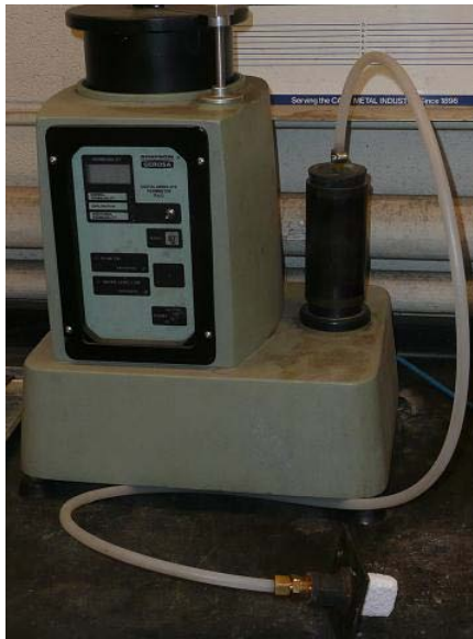
Figure 2.5 Digital permmeter with attached sample used to test mold permeability
