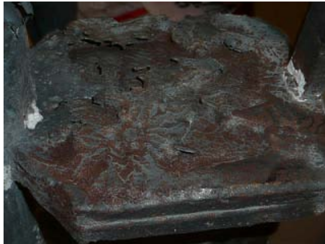
Figure 3.10 Top surface of the upper plate did not fill because air entrapment
