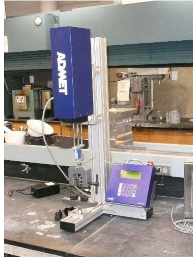
Figure 2.6 The flexural testing apparatus used to collect loading and displacement data
