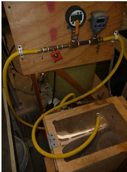
Figure 2.8 Burst test apparatus used to test internal pressure limits on three-dimensional samples.
