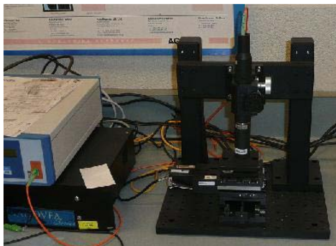
Figure 2.4 Nanovea Laser Surface Profiler used to measure surface quality of patterns, molds, and castings.
