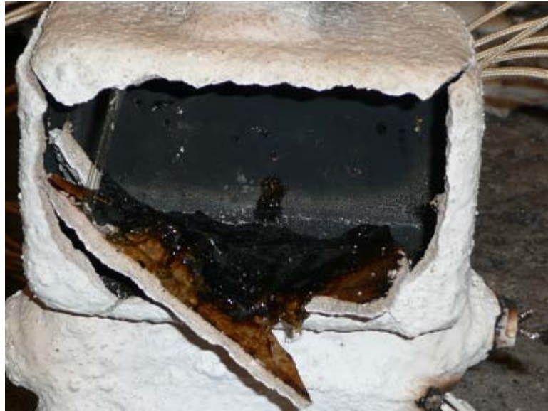
Figure 3.9 Pattern residues are observed inside of the mold that would not allow filling
