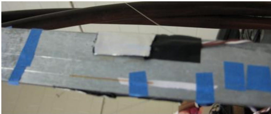
Figure 1.3. EFPI and strain gauge attached to steel structure
