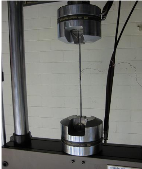
Figure 1.2. Strain measurement using EFPI sensor
