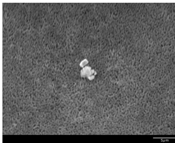
Figure 3.12. Cluster of particulate material collected on the 0.05 \mu\text{m} cellulose filter.
