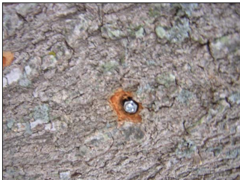
Figure B.4: SPS placed inside core space left after removal of the tree core
