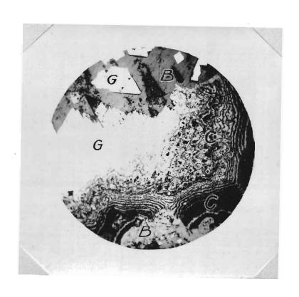
Figure 1. (75 x). Cerussite Replacing Galena.
