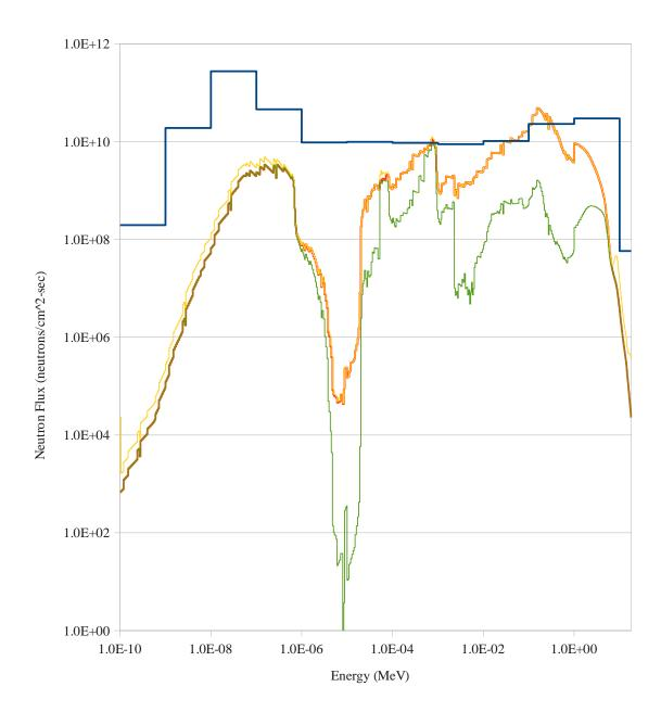
Fig. 7. Half Power neutron flux spectrum for the MSTR.
