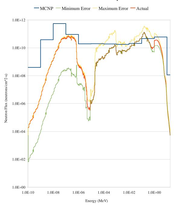
Fig. 6. Full Power neutron flux spectrum for the MSTR.
