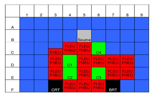
Fig. 1. Core configurations of the MSTR.
