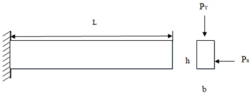
Figure 3.4 Cantilever beam example
