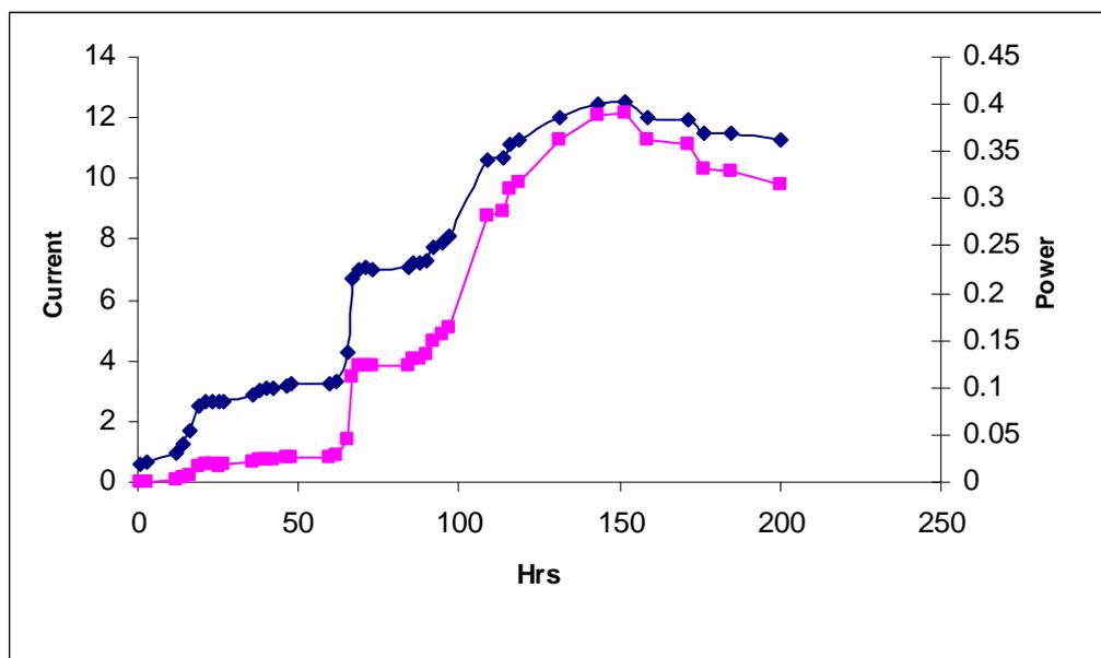
Figure 8. Current density (diamonds) in mA/m<sup>2</sup> and power density (squares) in mW/m<sup>2</sup> by using formate (30mM) as substrate.
