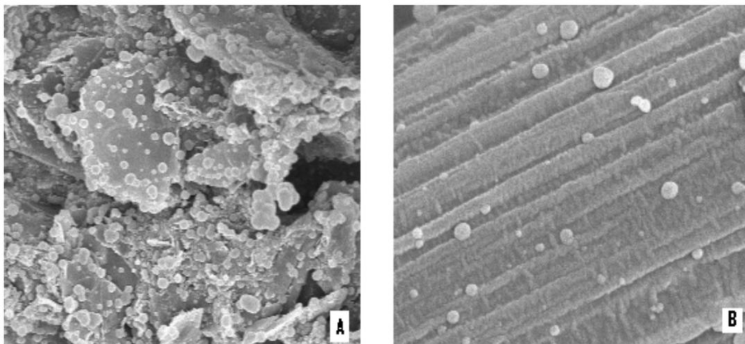
Figure 7. SEM image of reticulated carbon (A) and graphite carbon (B) materials (Original magnification: 2500X (A), 11000X (B)).
