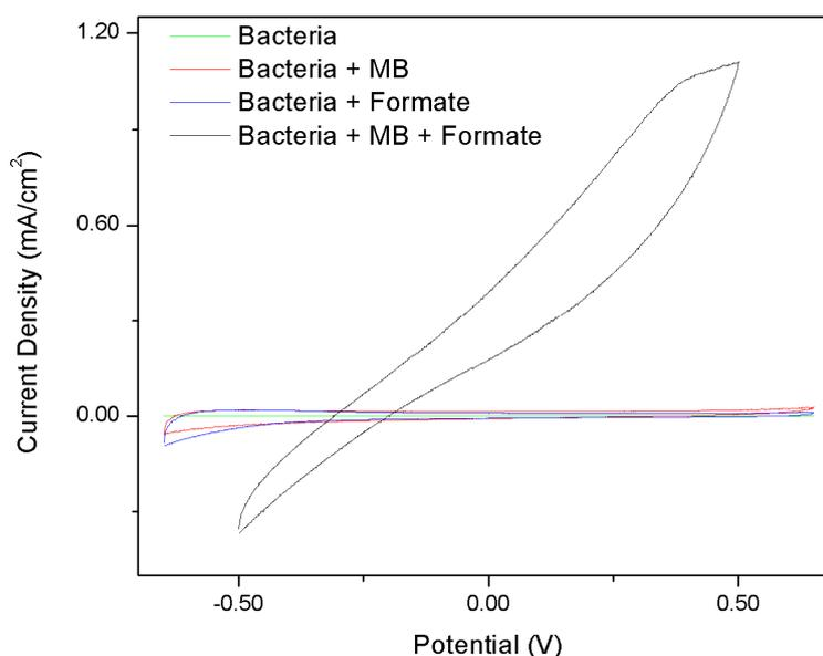
Figure 12. Cyclic voltammogram results obtained with different media components.
