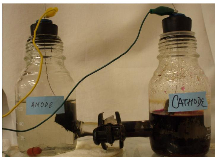
Figure 1. Dual-chambered MFC showing the anode and cathode chambers.
