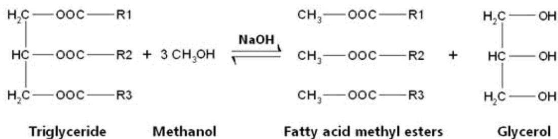
Figure 2.1. Transesterification reaction involving the conversion of triglycerides into biodiesel with the simultaneous production of glycerol.
