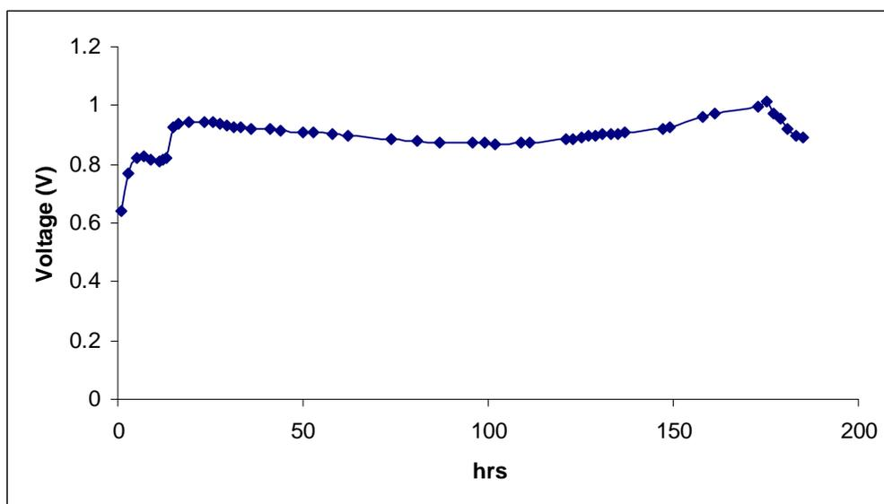
Figure 9. Open circuit voltage (in Volts) by using formate (30mM).
