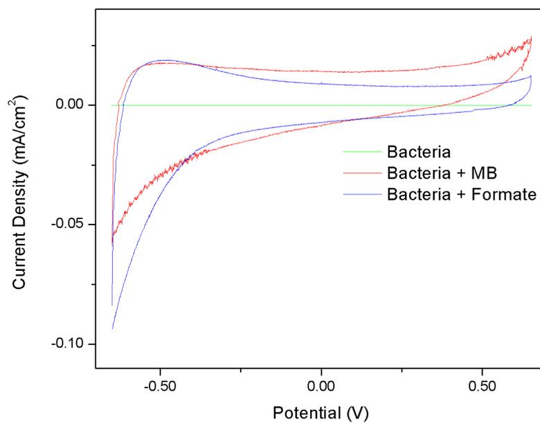
Figure 13. Cyclic voltammograms (enlarged results of bacteria, bacteria+MB and bacteria+formate).
