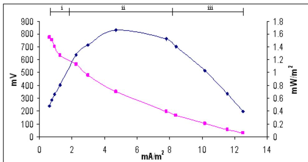
Figure 11. Polarization curve (squares) plot between current density and voltage and power curve (diamonds) plot between current density and power density. Sections i, ii, and iii represent the regions where different losses occur on the polarization curve.
