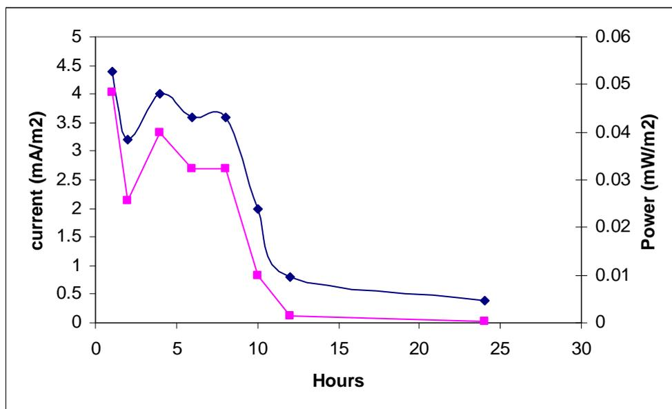
Figure 10. Current and power densities in MFC with no bacterial inoculation.
