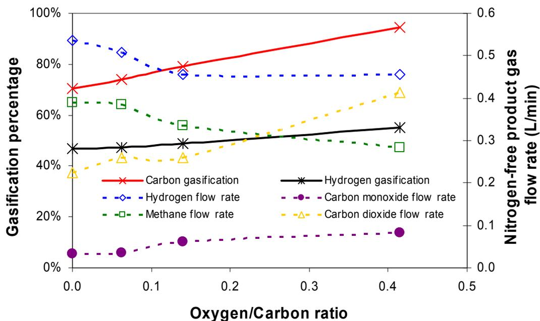
**Figure 5-3.** Nitrogen-free product gas flow rate and gasification percentage as a function of oxygen-to-carbon molar feed ratio. Experimental conditions,  $T = 764 \pm 2^\circ\text{C}$ ,  $P = 24.1 \pm 0.1 \text{ MPa}$ , space time =  $151 \pm 10 \text{ sec}$ .
