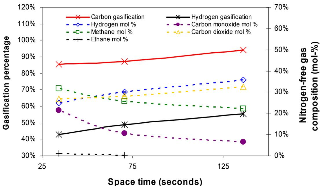
**Figure 5-2.** Nitrogen-free gas composition and gasification percentage as a function of space time. Experimental conditions,  $T = 764 \pm 1^\circ\text{C}$ ,  $P = 24.1 \pm 0.1 \text{ MPa}$ , oxygen to carbon ratio =  $0.411 \pm 0.009$ , aqueous aviation fuel concentration =  $6.2 \pm 0.3 \text{ wt } \%$ .
