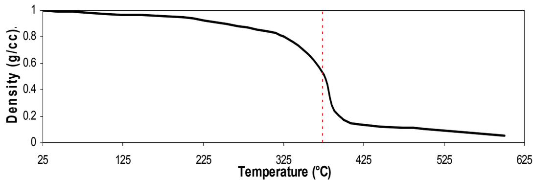
**Figure 2-3.** Density change of water as a function of temperature at a pressure of 3400 psi.<sup>31</sup>
