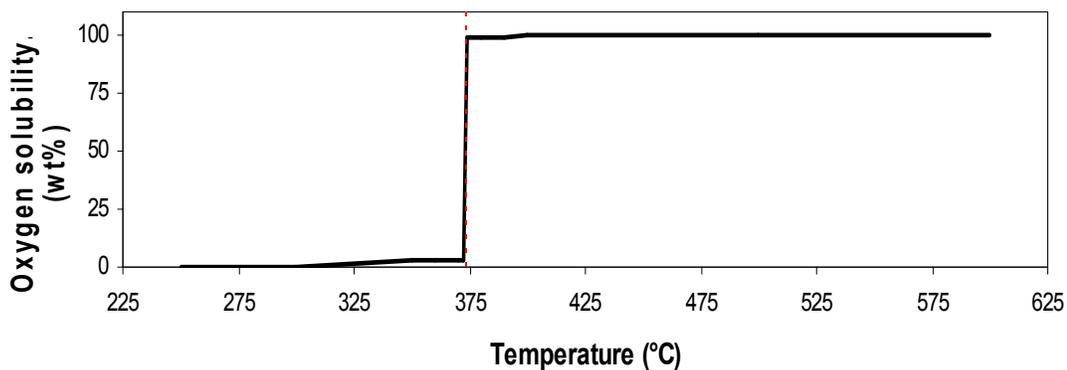
**Figure 2-4.** Oxygen solubility in water as a function of temperature at a pressure of 3400 psi.<sup>31</sup>
