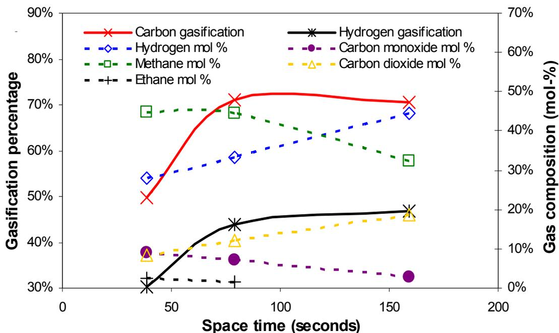
**Figure 5-1.** Total gas composition and gasification percentage as a function of space time. Experimental conditions,  $T = 770 \pm 2^\circ\text{C}$ ,  $P = 24.1 \pm 0.1 \text{ MPa}$ , aqueous aviation fuel concentration =  $6.1 \pm 0.4 \text{ wt } \%$ .
