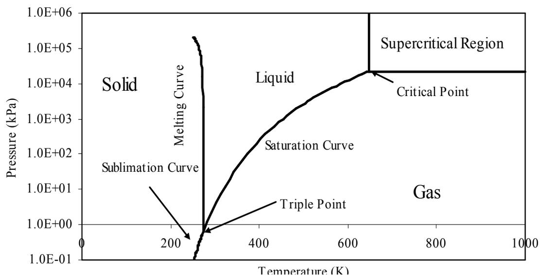
**Figure 2-2.** Phase diagram including supercritical region for water.
