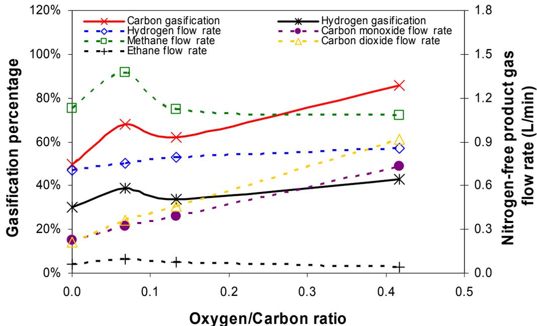
**Figure 5-5.** Nitrogen-free product gas flow rate and gaseous conversion as a function of oxygen- to-carbon molar feed ratio. Experimental conditions,  $T = 770 \pm 4^\circ\text{C}$ ,  $P = 24.16 \pm 0.03 \text{ MPa}$ , space time =  $37 \pm 2 \text{ sec}$ .
