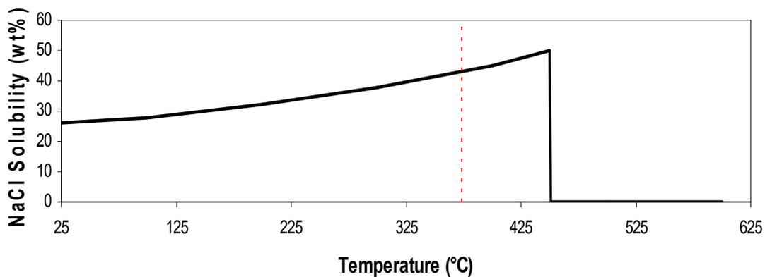
**Figure 2-5.** Sodium chloride solubility in water as a function of temperature at a pressure of 3400 psi.<sup>31</sup>
