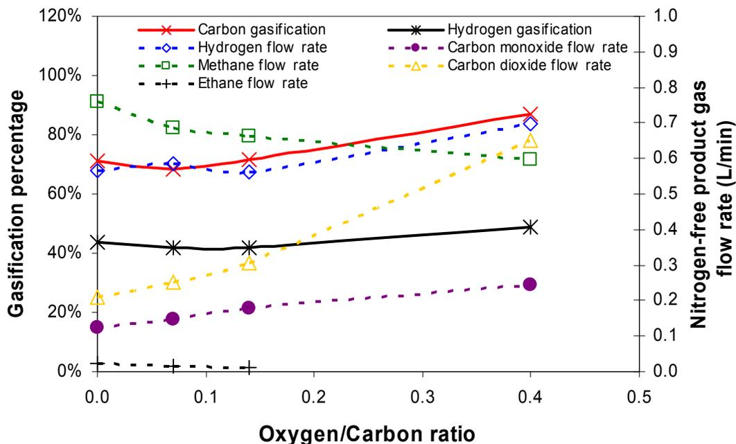
**Figure 5-4.** Nitrogen-free product gas flow rate and gaseous conversion as a function of oxygen-to-carbon molar feed ratio. Experimental conditions,  $T = 770 \pm 3^\circ\text{C}$ ,  $P = 24.1 \pm 0.1$  MPa, space time =  $75 \pm 4$  sec.
