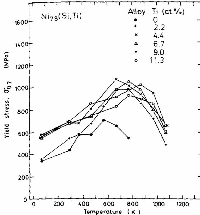
Figure 1.3 The dependence of titanium concentration on the mechanical strength of  $Ni_3(Si,Ti)$  [1].
