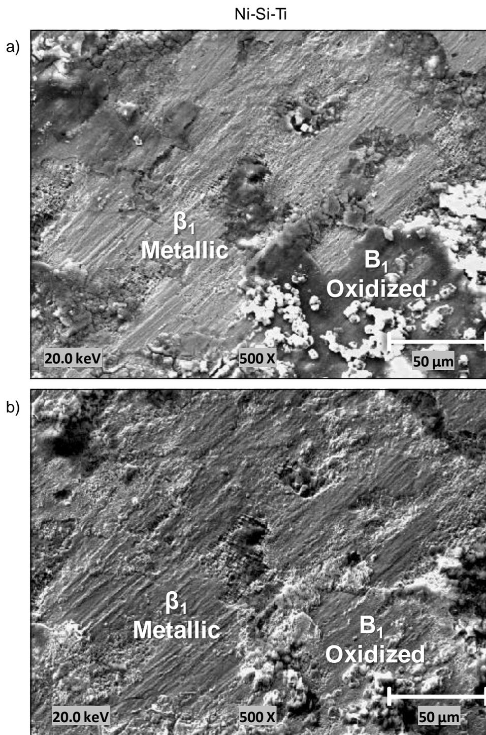
**Figure 8** BSE images taken a) before, and b) after sputter profiling of a Ni-Si-Ti alloy surface that was corroded in boiling 70 wt. % sulfuric acid for one minute. Auger composition maps of the oxidized and metallic  $\beta_1$  phases labeled in this figure are shown in Figure 9.
