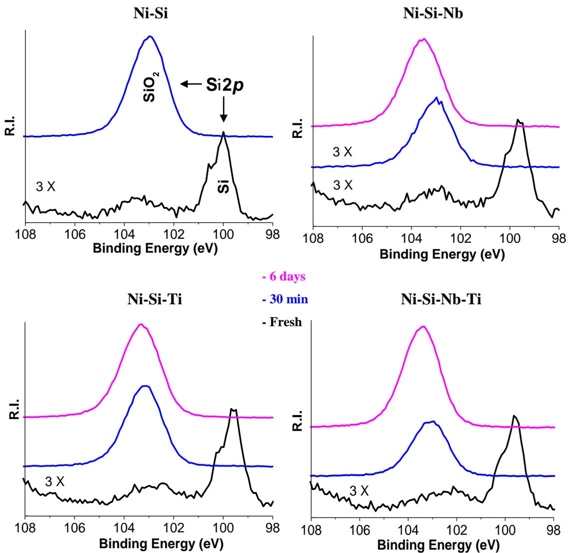
Figure 3.29 High resolution Si 2p spectra taken from Ni<sub>3</sub>Si alloys following exposure to boiling 70 wt. % sulfuric acid
