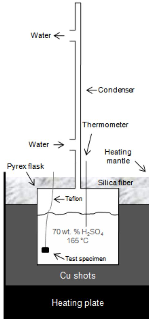
Figure 2.1 Corrosion testing apparatus used for corrosion experiments.
