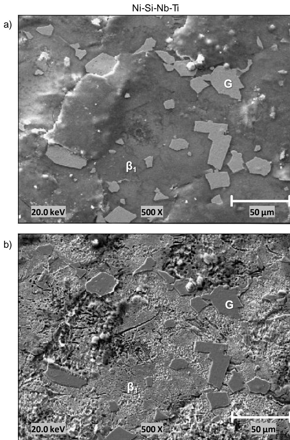
**Figure 6** BSE images taken a) before, and b) after sputter profiling of a Ni-Si-Nb-Ti alloy surface that was corroded in boiling 70 wt. % sulfuric acid for one minute. Auger composition maps of the  $\beta_1$  and G phases labeled in this figure are shown in Figure 7.
