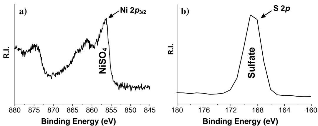
Figure 3.28 High resolution a) Ni 2p and b) S 2p photoelectron spectra of nickel sulfate.
