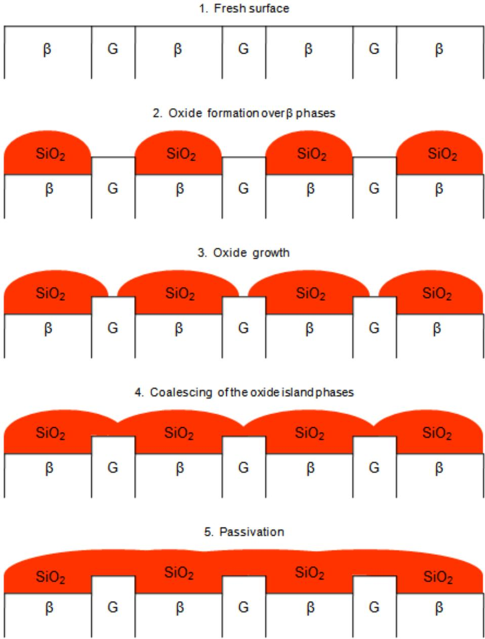
Figure 4.1 The corrosion process of Ni<sub>3</sub>Si alloys in boiling 70 wt. % sulfuric acid.
