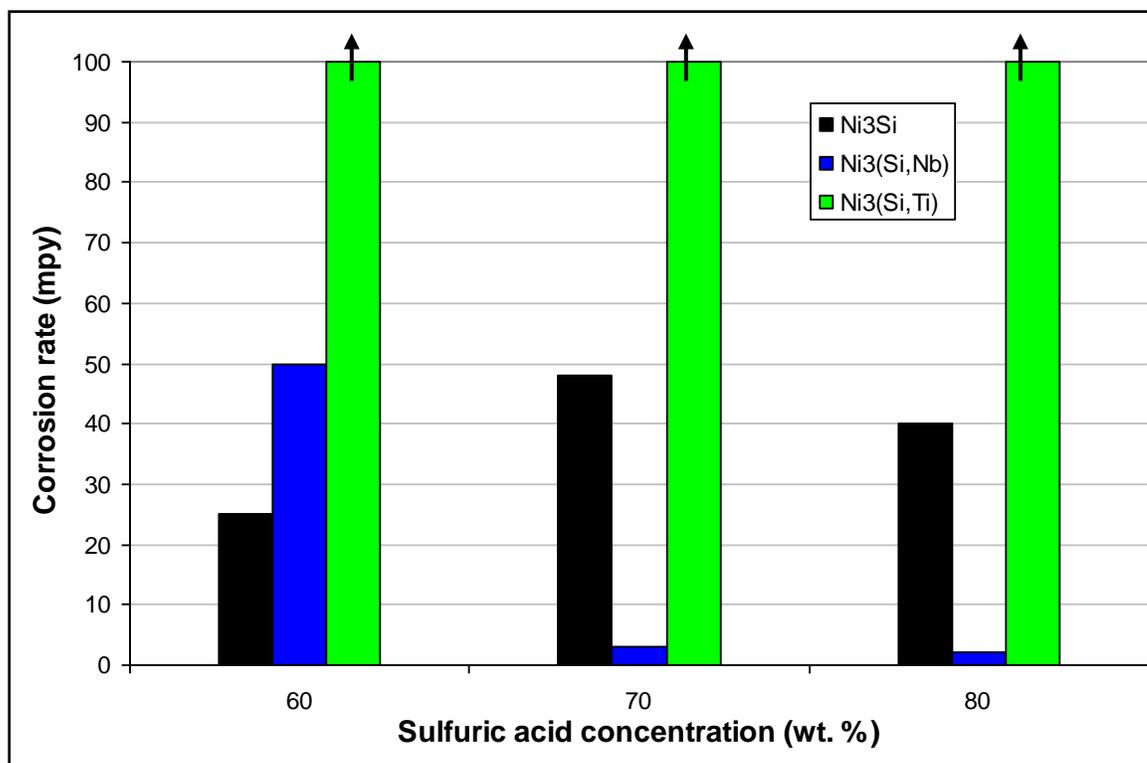
Figure 1.7 The corrosion rates of Ni<sub>3</sub>Si alloys in boiling sulfuric acid [2].
