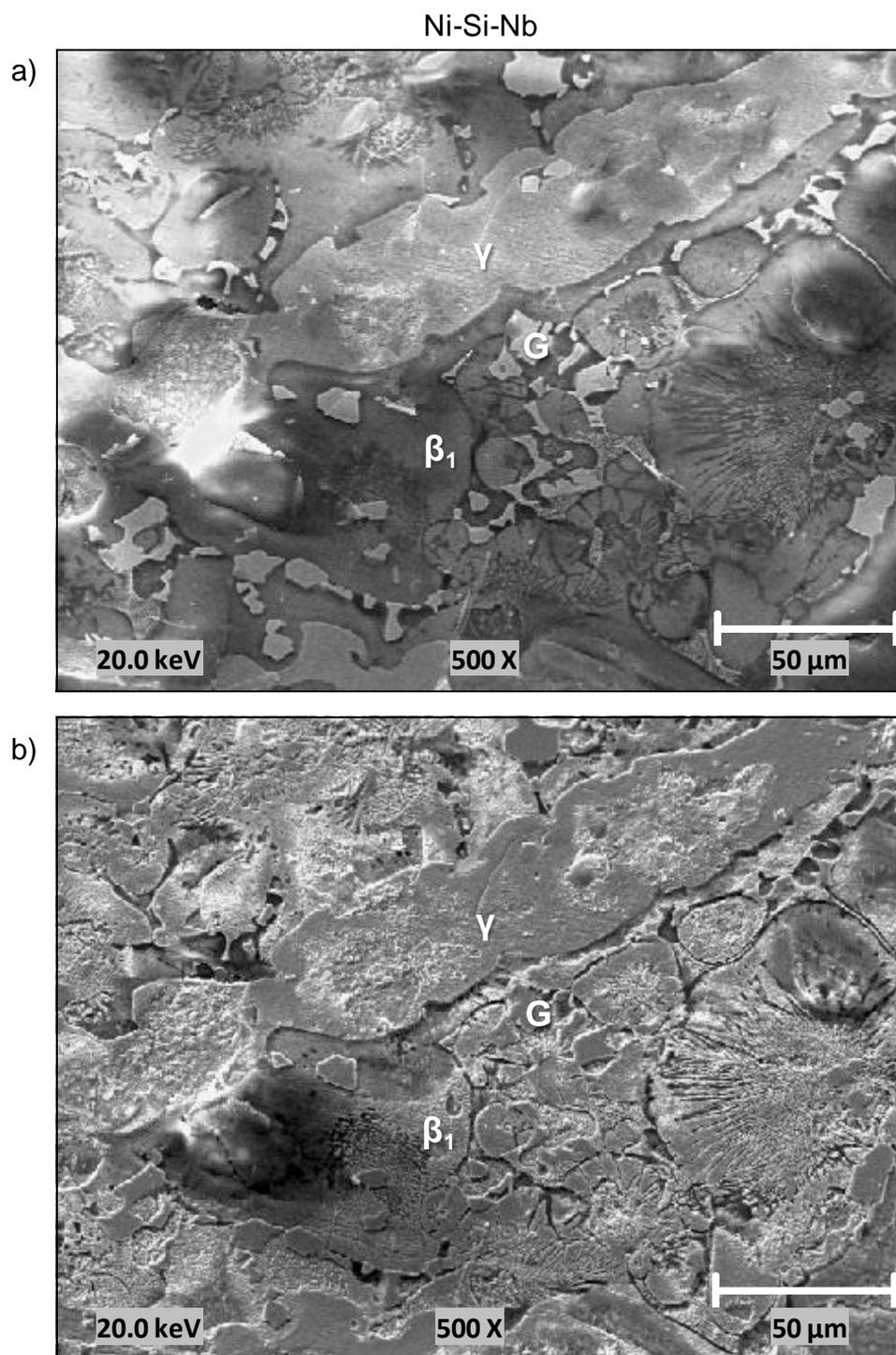
**Figure 4** BSE images taken a) before, and b) after sputter profiling of a Ni-Si-Nb alloy surface that was corroded in boiling 70 wt. % sulfuric acid for one minute. Auger composition maps of the  $\beta_1$ ,  $\gamma$ , and G phases labeled in this figure are shown in Figure 5.
