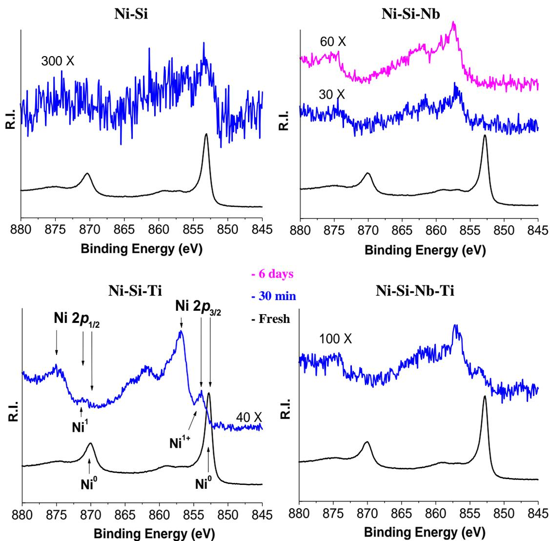
Figure 3.26 High resolution Ni 2p spectra of Ni<sub>3</sub>Si alloy surfaces following exposure to boiling 70 wt. % sulfuric acid.
