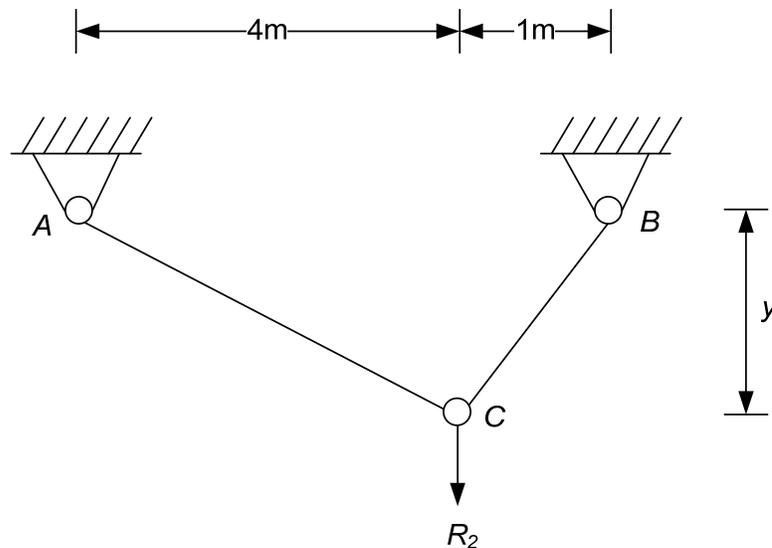
Figure 6.1. A Two-Bar Pin Jointed Truss Problem
