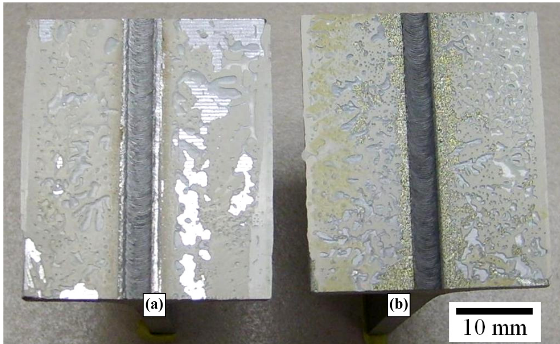
Figure 3.11. T-rail of failed sealed welds with (a) no prior anodization and with (b) prior standard sulfuric acid anodization. (b) shows evidence of anodized layer delamination from the top-skin.
