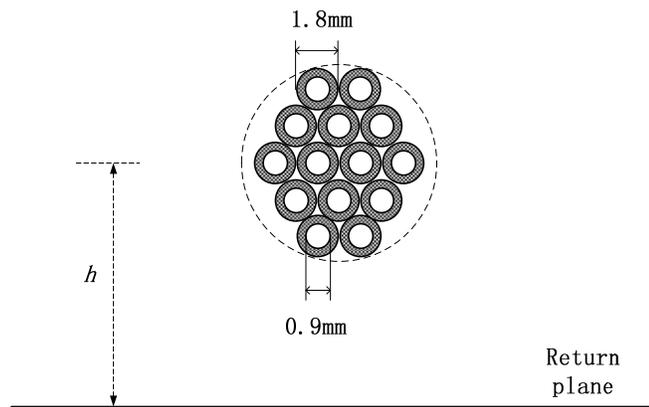
Figure 1.1. Cross section of a 14 wire harness
