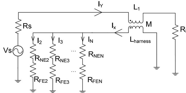
Figure 1.7. Circuit model approximating strong inductive coupling
