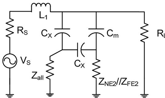
Figure 1.8. Circuit model approximating strong capacitive coupling
