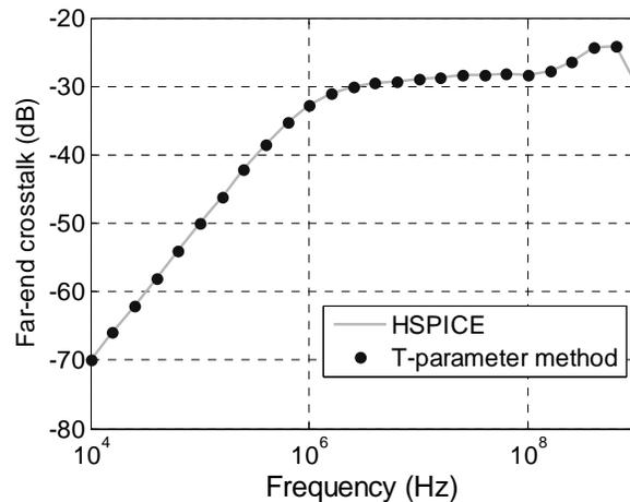
Figure 2.6. Comparison of the simulation results for far-end crosstalk from circuit 2 to circuit 1 for a 14-wire bundle when all wires are loaded with 50 ohm at both ends
