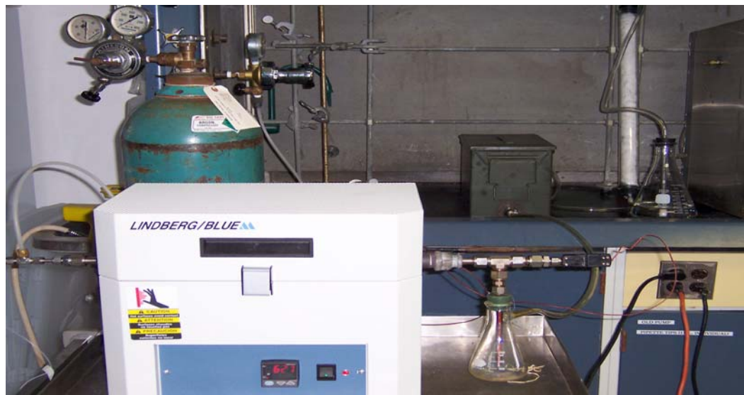
Figure 3.3. A photograph of the oil volatilization and condensation set-up. Adapted from "Evaluations of antimicrobial activities of volatiles produced during rapid volatilization of oils"
