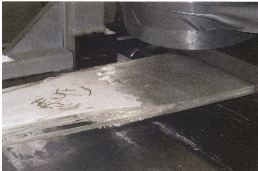
Figure 2.15. Cured Core-filled Pultruded Part
