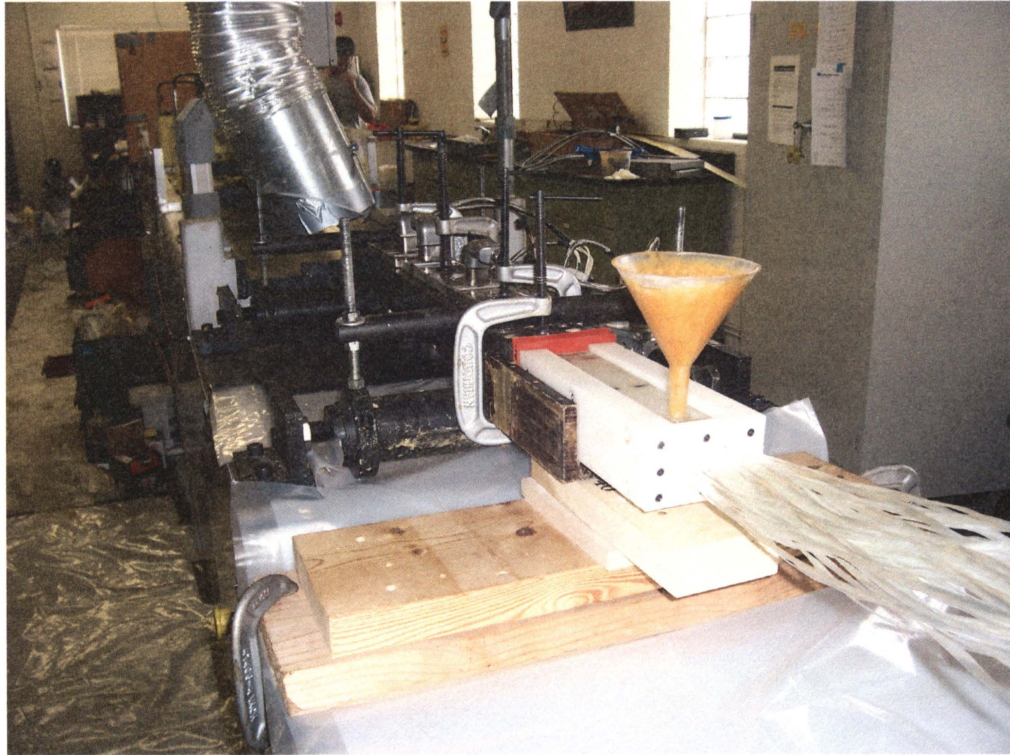
Figure 2.1. Setup for the PU Pultrusion at UMR
