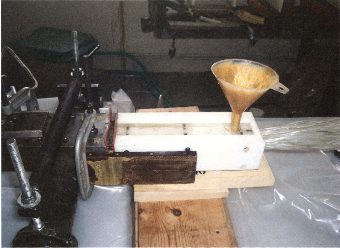
Figure 2.3. Injection Box and the Pultrusion Die Connected with a Connector
