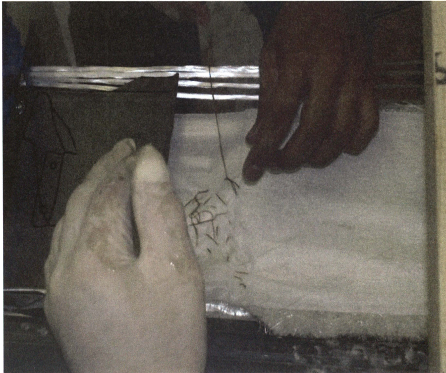
Figure 2.14. Stitching Mat and Veil with Rovings
