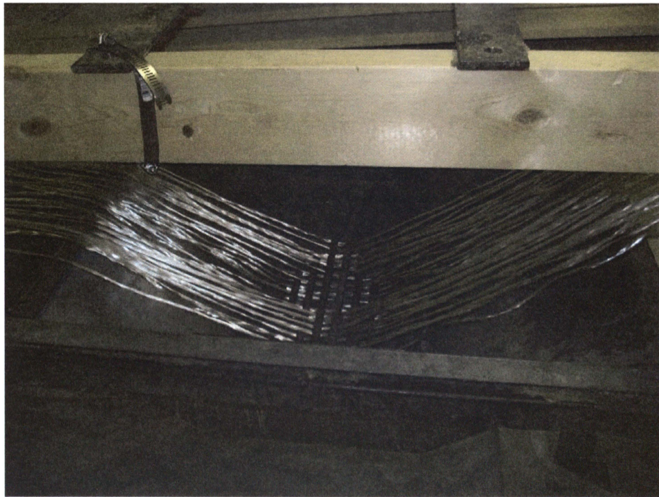
Figure 2.7. Fiber Placement in the Resin Bath
