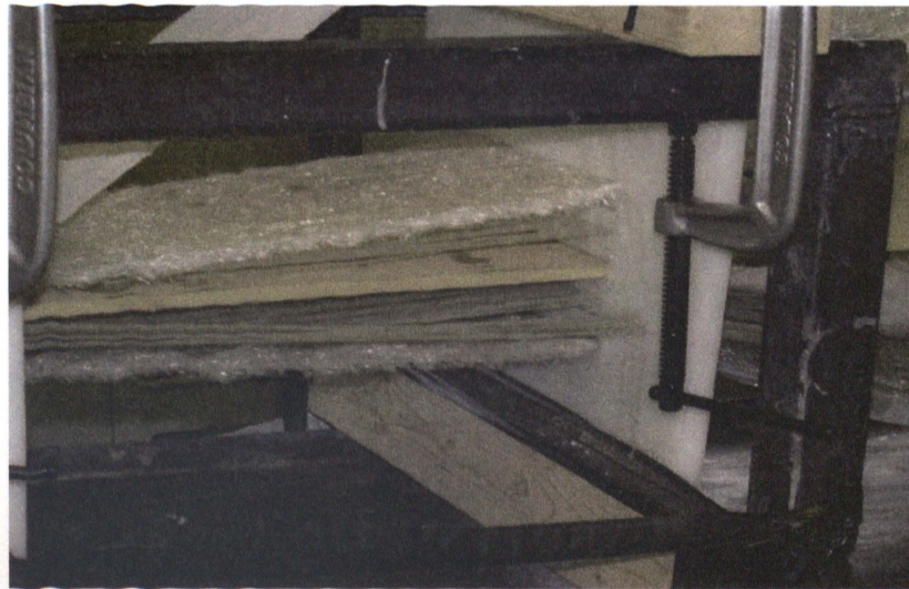
Figure 2.10. Arrangement of Mat, Fiber and Core in Preform 1
