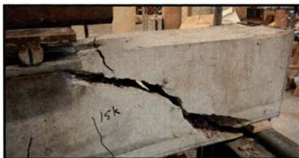
Figure 4.3. Shear Failure Pattern
