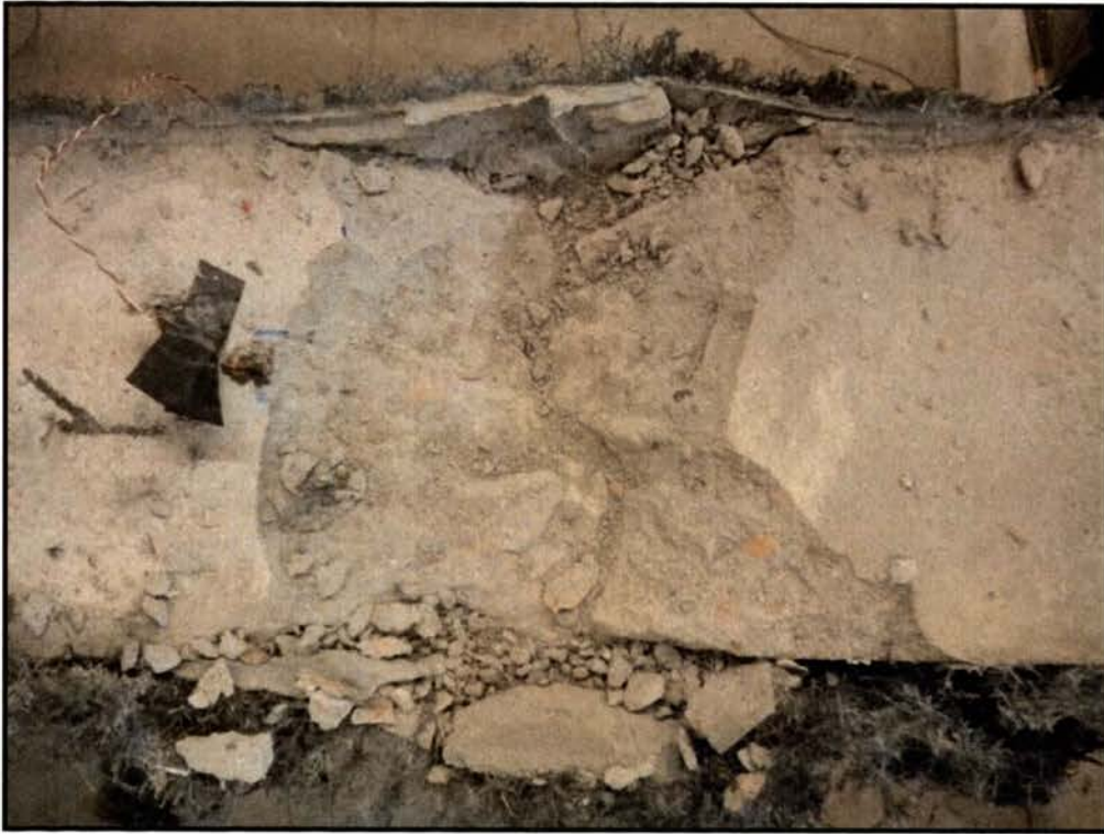
Figure 4.7. Top View of Failed Test Beam SR-P-A-L
