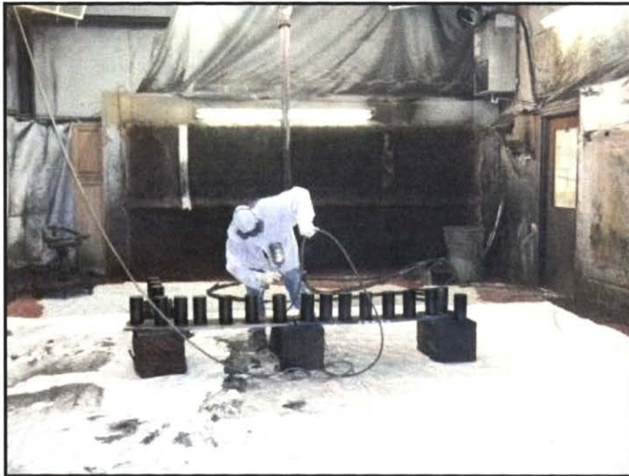
Figure 3.3. Priming of Concrete Cylinders
