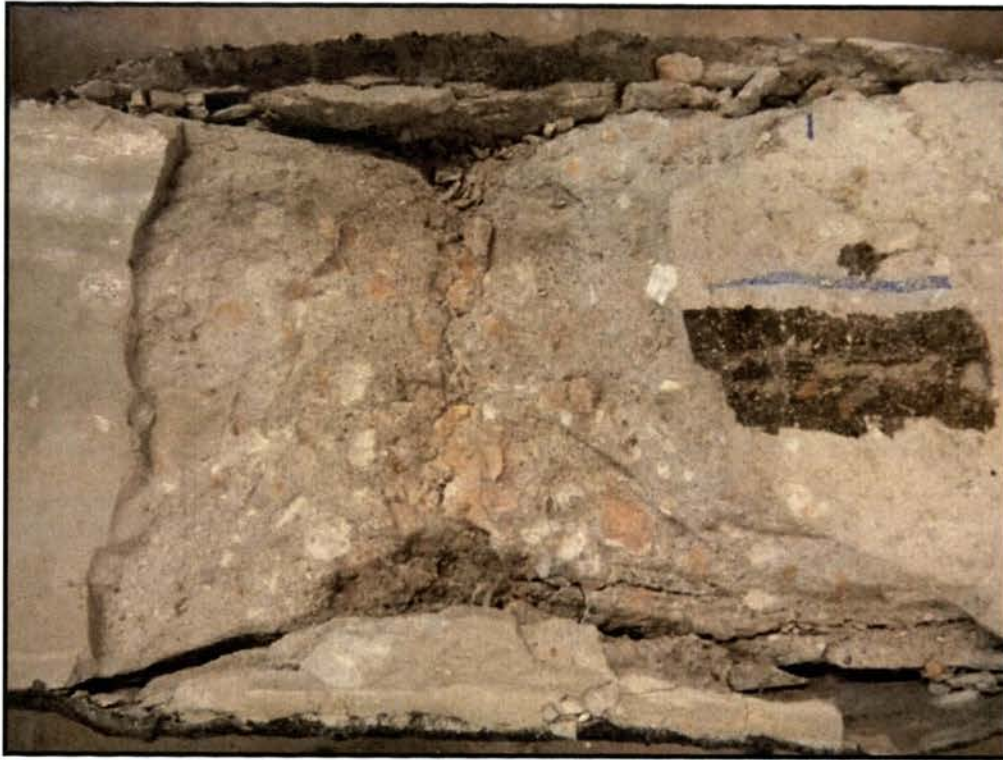
Figure 4.11. Top View of Failed Test Beam F-P-A-0
