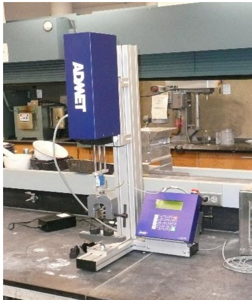
Figure 3.16. ADMET Universal Testing Apparatus for three-point bend test
