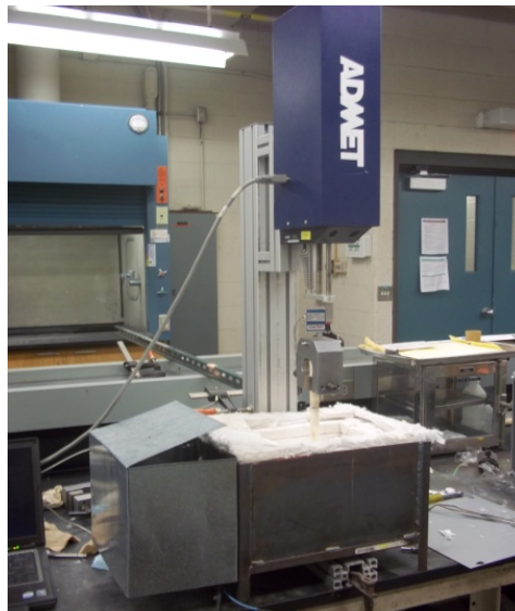
Figure 3.17. Furnace chamber attached to ADMET machine for high temperature testing
