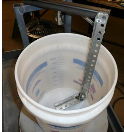
Figure 3.14. Setup for slurry mixing
