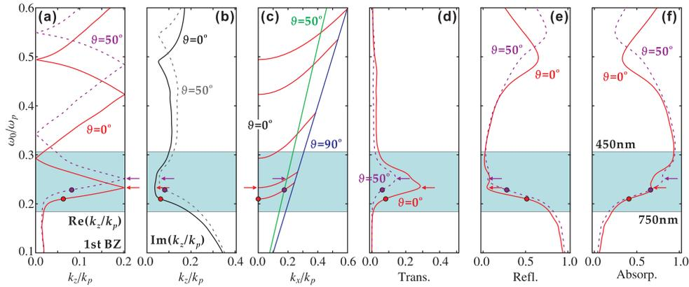
Fig. 2. (a) The real part and (b) the imaginary part of the band structure of the Au-Al<sub>2</sub>O<sub>3</sub> multilayer stack. (c) The dispersion relation of the Au-Al<sub>2</sub>O<sub>3</sub> multilayer stack. (d) The transmission, (e) reflection, and (f) absorption spectra of the Au-Al<sub>2</sub>O<sub>3</sub> multilayer stack.
