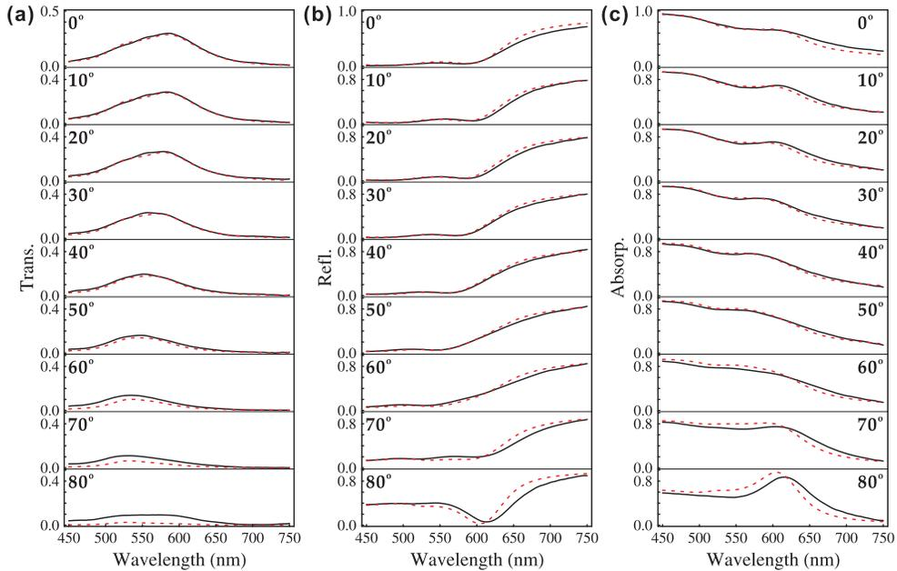
Fig. 3. (a) The transmission, (b) reflection, and (c) absorption spectra of the Au-Al<sub>2</sub>O<sub>3</sub> multilayer stack in experiments (black curves) and in theory (red curves) at different angles of incidence from 10° to 80°.
