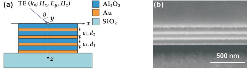
Fig. 1. (a) Schematic of the Au- $\text{Al}_2\text{O}_3$  multilayer stack on a quartz substrate. (b) The SEM picture of the cross section of the fabricated 4-pair Au- $\text{Al}_2\text{O}_3$  multilayer stack.
