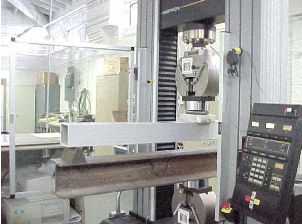
Figure 8: Testing of hollow composite tube using Instron 4485 machine.
