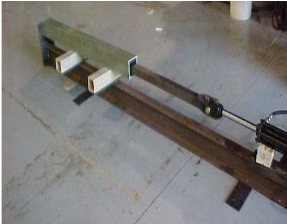
Figure 6: Tube-filling machine spine and ram when fully extended.
