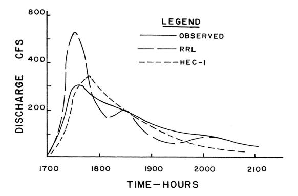
FIGURE 5. - RRL VS. OBSERVED PEAK DISCHARGES
