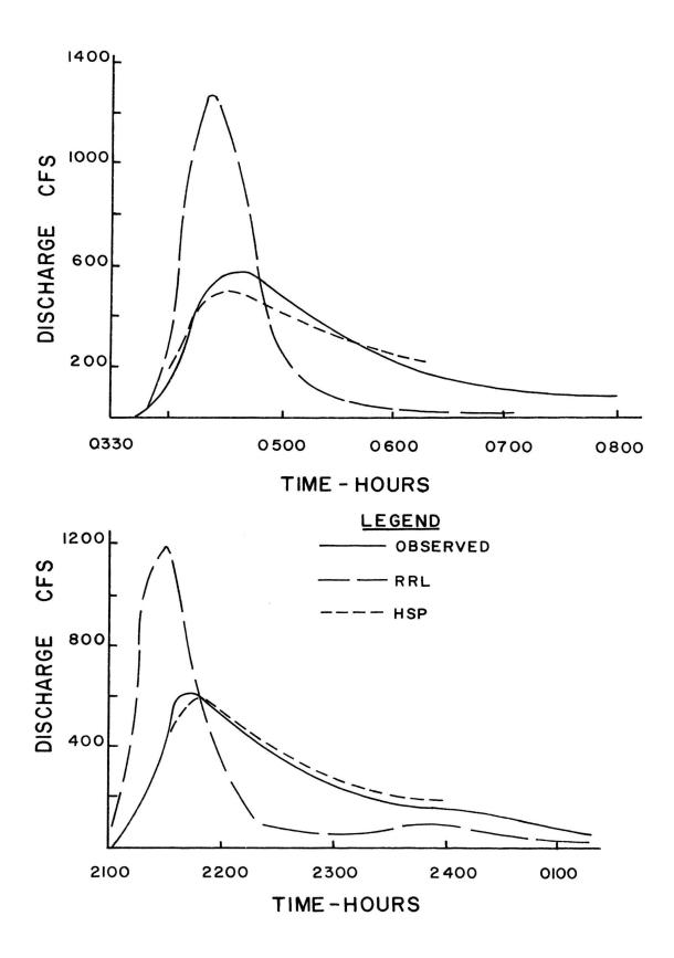
FIGURE 9. - RRL VS. OBSERVED PEAK DISCHARGES
