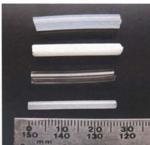
Figure 2 - Photograph showing the SPSs used in testing (to scale). (From top to bottom) Polydimethylsiloxane (PDMS) tubing, polyoxymethylene (POM) rod, polyvinylchloride (PVC) tubing and low density polyethylene (LDPE) tubing.
