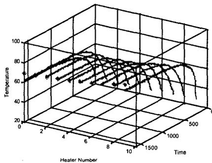
Figure 5: Temperature history for desired parabolic profile
