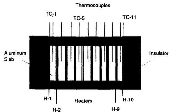
Figure 1: Cross section of experimental setup
