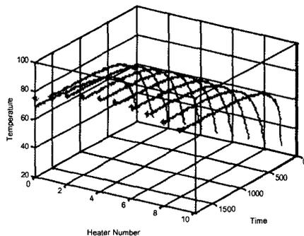
Figure 7: Temperature history for desired parabolic profile
