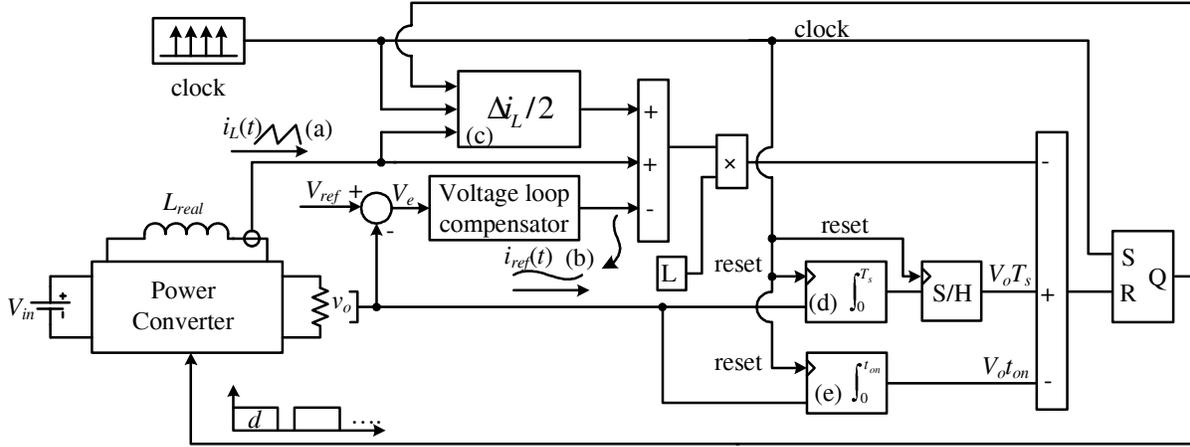
Figure 6. Block diagram of PCPC approach.
