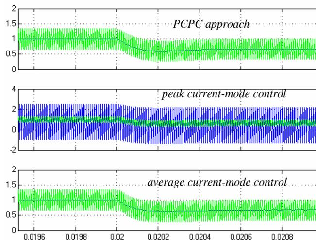
Figure 12. Inductor current and its reference waveforms when load changes from 2  $\Omega$  to 3  $\Omega$  at 0.02 s.
