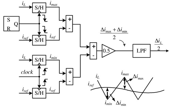
Figure 7. Block diagram of the steady-state peak-to-peak ripple finder.
