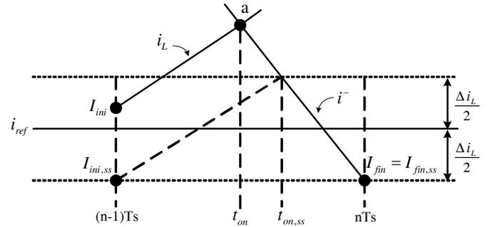
Figure 5. Typical current waveform of a buck converter.
