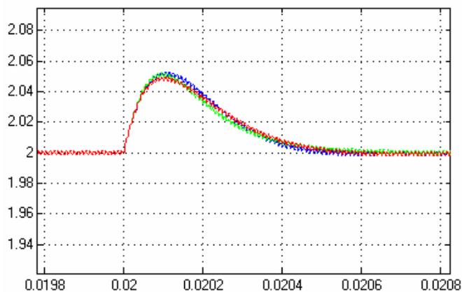
Figure 11. Output voltage waveforms when load changes from 2  $\Omega$  to 3  $\Omega$  at 0.02 s.
