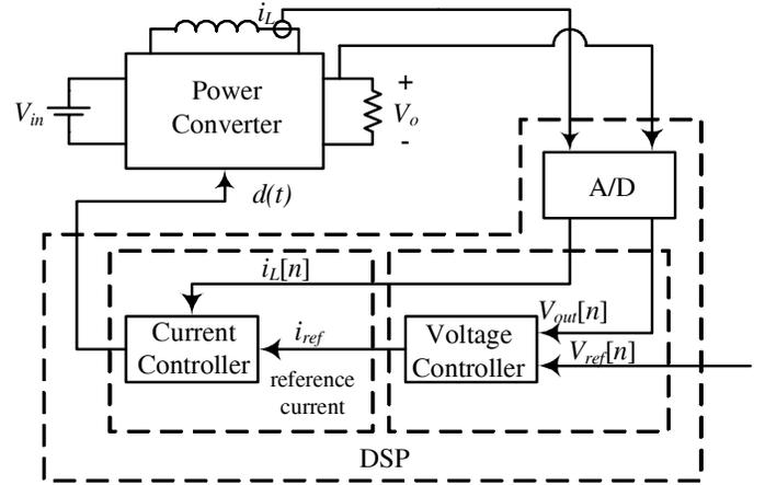
Figure 4. Block diagram of the digital current-mode controller.
