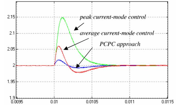
Figure 9. Transients in the output voltage when input voltage  $V_{in}$  changes from 3 V to 6 V at 0.01 s.
