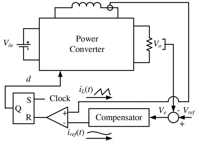
Figure 1. Block diagram of a peak current-mode controller.
