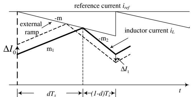
Figure 3. Propagation of a perturbation in the presence of a suitable ramp (Stability can be maintained for all  $d$ ).
