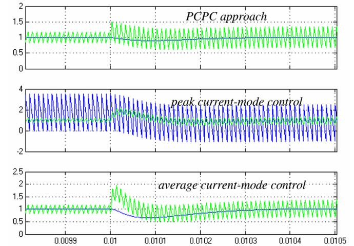
Figure 10 Inductor current and its reference waveforms when  $V_{in}$  changes from 3 V to 6 V at 0.01 s.
