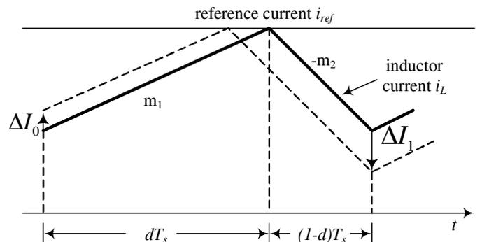
Figure 2. Propagation of a perturbation when  $d$  is greater than 0.5.
