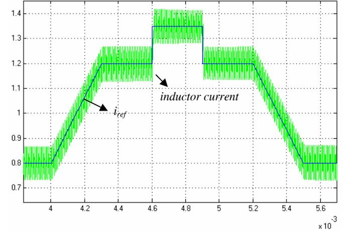
Figure 8. The inductor current waveform using PCPC approach.
