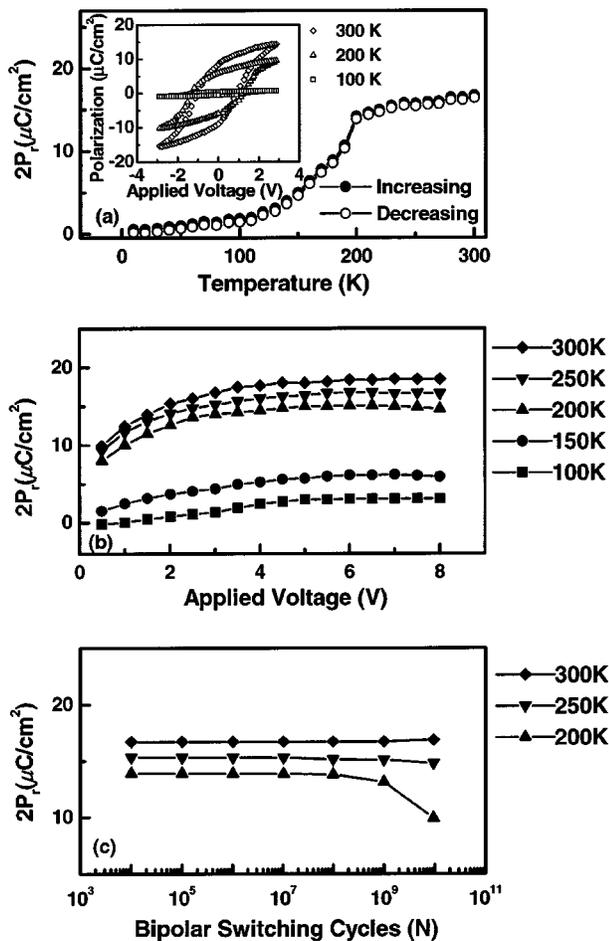
FIG. 1. The temperature dependence of twice the remanent polarization ( $2P_r$ ) of SBT thin films: (a)  $2P_r$  at 3 V for both decreasing temperature (open), increasing temperature (solid), and the hysteresis loop at variable temperature (inset) and (b)  $2P_r$  vs voltage at various temperature; and (c) the fatigue behavior of  $2P_r$  as a function of temperature at 3 V bipolar pulse with 1 kHz.
