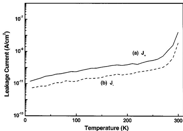
FIG. 4. Temperature dependence of the leakage current of a Pt/SBT/Pt sample at 3 V: (a)  $J_+$  and (b)  $J_-$  are leakage currents with the top electrode positively and negatively biased, respectively.
