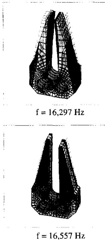
Figure 3: The lowest two resonant frequency modes of the final design of the miniature tuning fork motor with open-circuited piezoelectric material
