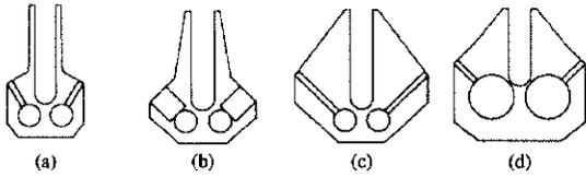
Figure 2: Result of changing the geometry through its parameters; (a) an increase in  $\theta$  from  $45^\circ$  to  $60^\circ$ , (b) an increase in  $n_{PZT}$  from two to eight, (c) an increase in  $w_{PZT}$  from 25 to 50, and (d) an increase in  $r_H$  from 10 to 20
