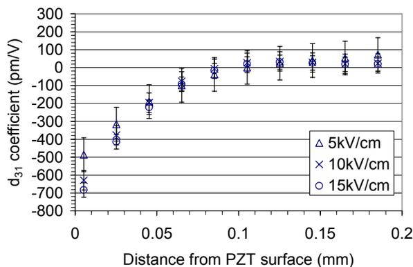
Figure 5. Distribution of piezoelectric  $d_{31}$  coefficient throughout the thickness of the 6-mil substrate device expressed by the 3<sup>rd</sup> order polynomial equations.
