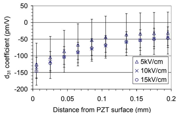
Figure 6. Distribution of piezoelectric  $d_{31}$  coefficient throughout the thickness of the 20-mil substrate device expressed by the 3<sup>rd</sup> order polynomial equations.
