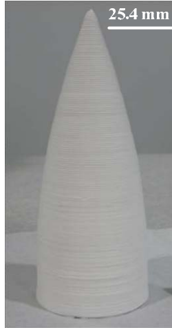
Figure 22: Large ogive cone fabricated with extrusion force controller.
