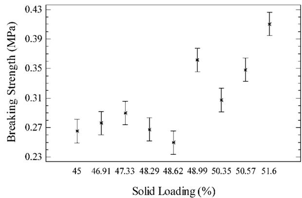
10 Effect of solids loading on breaking strength
