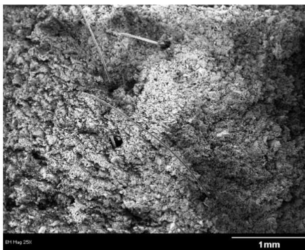
13 Scanning electron microscopy image of ceramic mould showing evidence of fibre pullout
