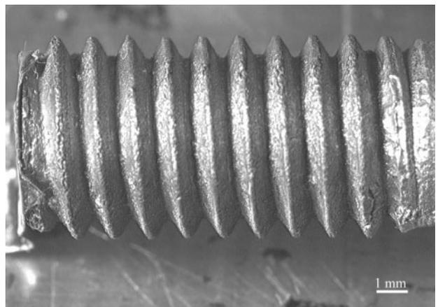
**15 Threads of metal casting for M8 bolt**
