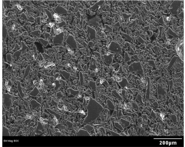
**14 Microstructure of fired test bar**
