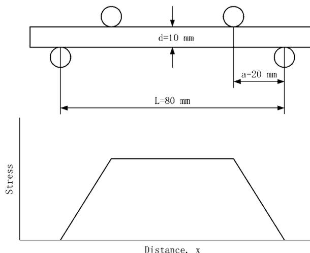
4 Stress distribution in four point bend testing
