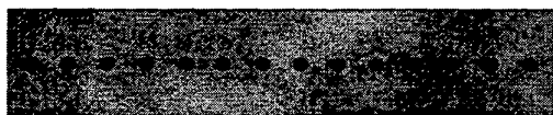
Figure 2: Horizontal Shadowgraph of the Backlit Stream of Droplets Perturbed by the Conventional Sinusoidal Disturbance.
