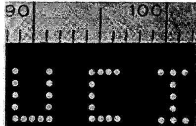
Figure 12: Mottened solder splats composing the characters "UCI"
