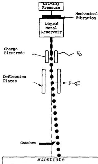
Figure 1: Schematic of Continuous Solder Droplet Printing.
