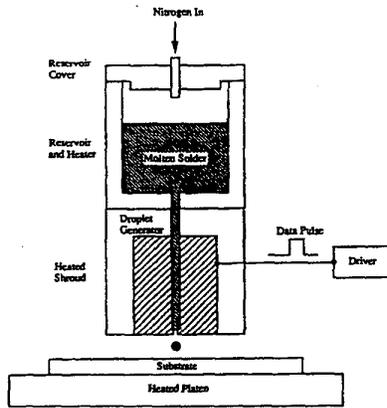
Figure 2: Schematic of Drop-on-demand Printing System
