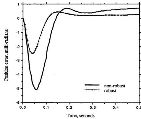
Fig. 8. Time histories of position error for the robust and nonrobust controllers using estimated acceleration measurements,  $-40\%$  error in payload inertia, and  $+30\%$  error in motor resistance. The robust control parameters are:  $\pi = 10^{10}$ ,  $\delta q_1 = \delta q_2 = 0.35$ ,  $\Delta f_4 = \Delta f_5 = 10^{-5}$ .
