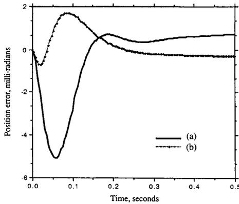
Fig. 7. Time histories of position error along the cubic trajectory using estimated acceleration measurements: (a)  $-40\%$  error in inertia and  $+30\%$  error in motor resistance; (b)  $+40\%$  error in inertia and  $-30\%$  error in motor resistance.
