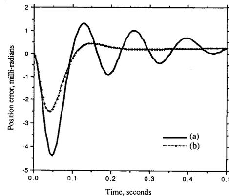
Fig. 9. Time histories of position error for the robust controller using estimated acceleration measurements,  $-40\%$  error in payload inertia, and  $+30\%$  error in motor resistance: (a)  $\pi = 1$ ,  $\delta q_1 = \delta q_2 = 0.35$ ,  $\Delta f_4 = \Delta f_5 = 10^{-5}$ ; (b)  $\pi = 10^{10}$ ,  $\delta q_1 = \delta q_2 = 0.35$ ,  $\Delta f_4 = \Delta f_5 = 10^{-5}$ .
