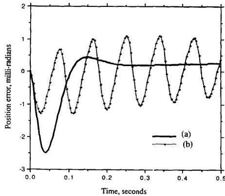
Fig. 10. Time histories of position error for the robust controller with various error bound sizes  $\phi$ : (a)  $\pi = 10^{10}$ ,  $\delta q_1 = \delta q_2 = 0.35$ ,  $\Delta f_4 = \Delta f_5 = 10^{-5}$ ; (b)  $\pi = 10^{10}$ ,  $\delta q_1 = \delta q_2 = 0.75$ ,  $\Delta f_4 = \Delta f_5 = 10^{-5}$ .
