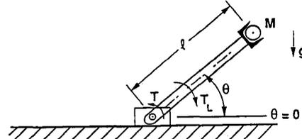
Fig. 2. Direct-drive arm actuated by a BLDCM.  $l = 1.0$  m,  $M = 2.0$  kg. The link is assumed massless.
