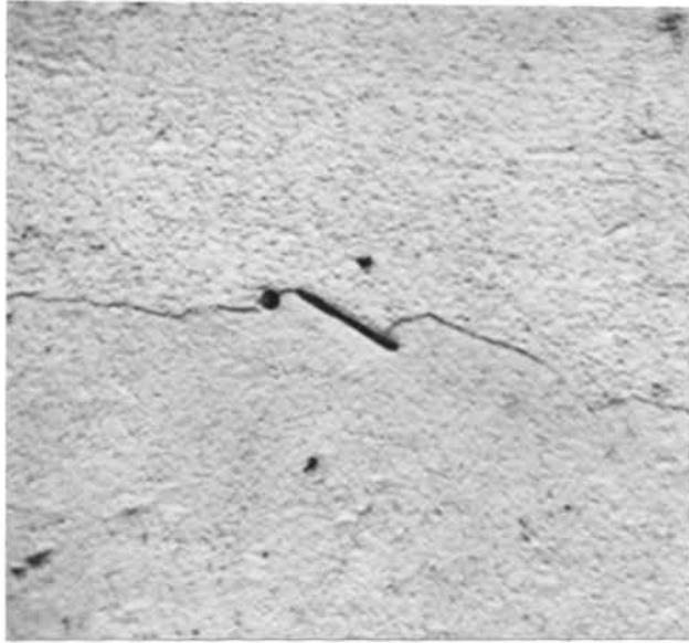
Figure 3. Plate-shaped allotriomorph in Pb-3.0 wt% Sn alloy after 53 hours of aging at 23°C. Apparent replacive motion by the grain boundary as reported by Tu and Turnbull. (7) X500
