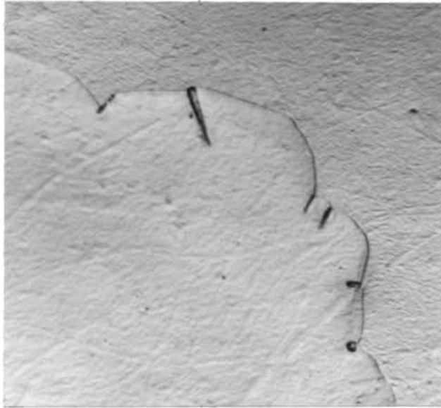
Figure A-2. \beta tin lamellae developing at edge of the cell. Note the different directions of the lamellae. Pb-3.0 wt% Sn alloy aged for 362 hours at 34°C. X500
