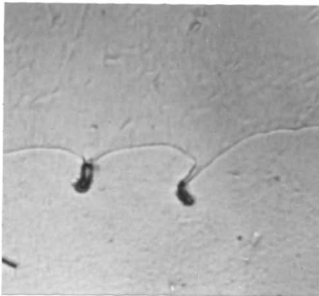
Figure 6. Formation of the \beta tin lamellae during the early stage of cell development of the Pb-3.0 wt% Sn after 76 hours aged at 23°C. Note the large bowing of the \alpha'/\alpha_2 boundary and the non habit orientation of the \beta tin lamellae. X2000
